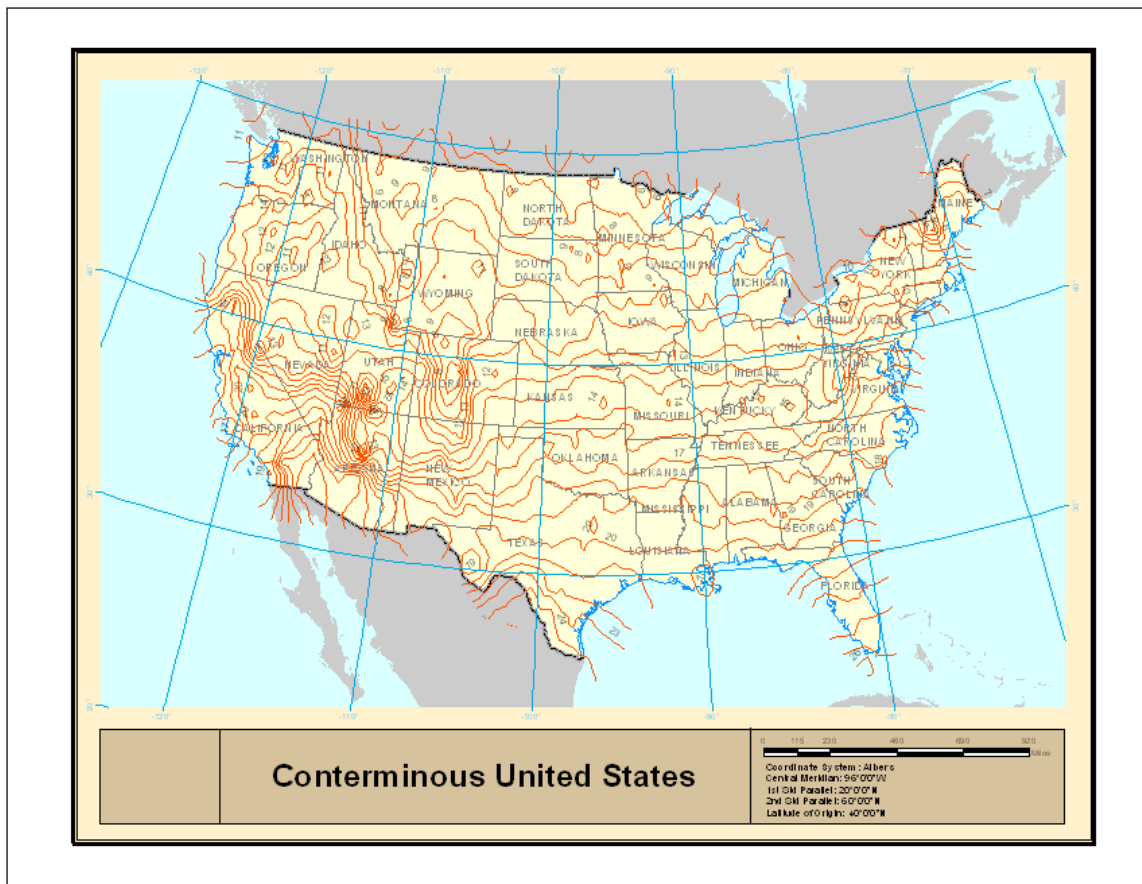
Figure B-1: Annual average ground temperature for Continental US, short grass covered sites
