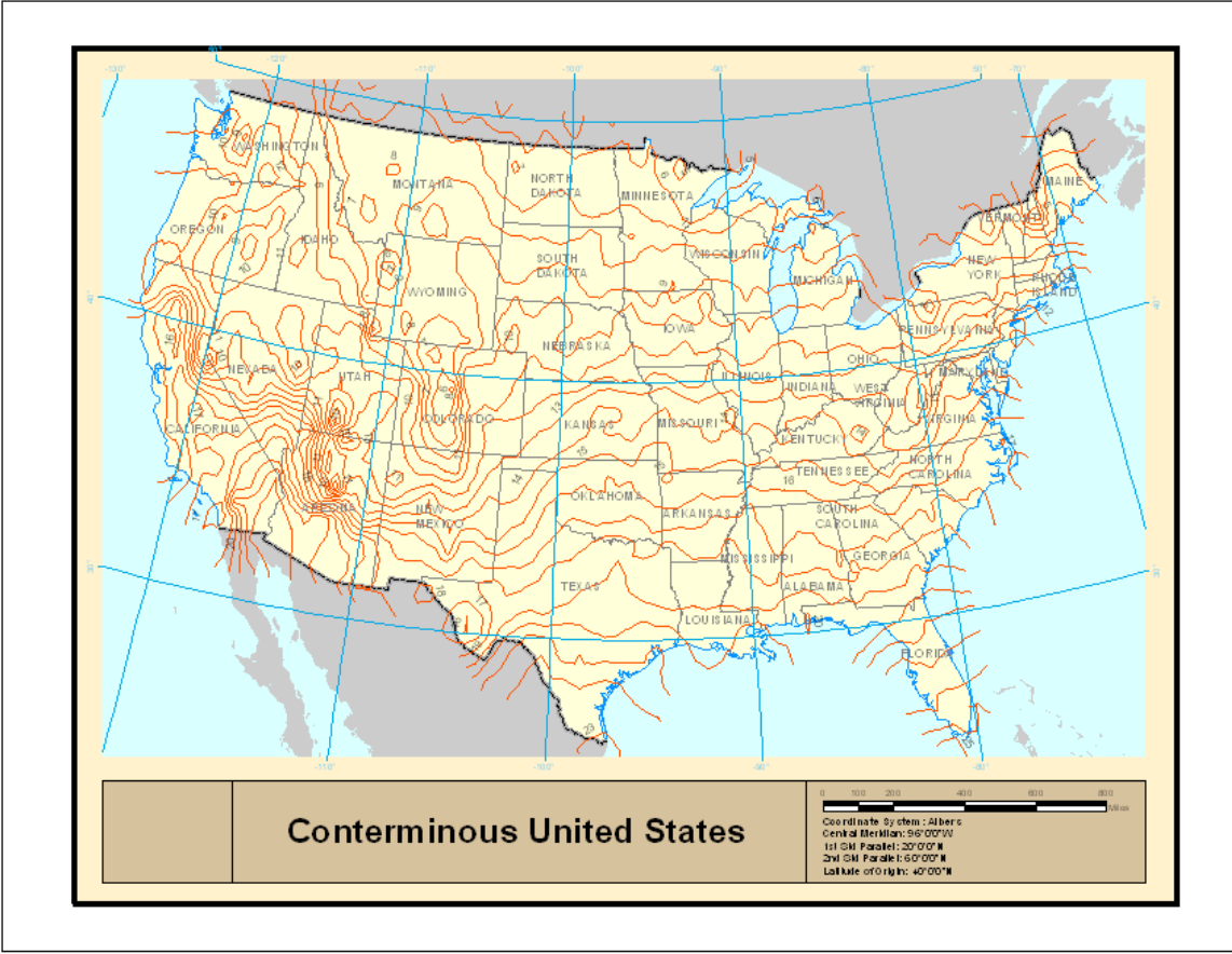
Figure B-13: Annual average ground temperature for Continental US, tall grass covered sites
