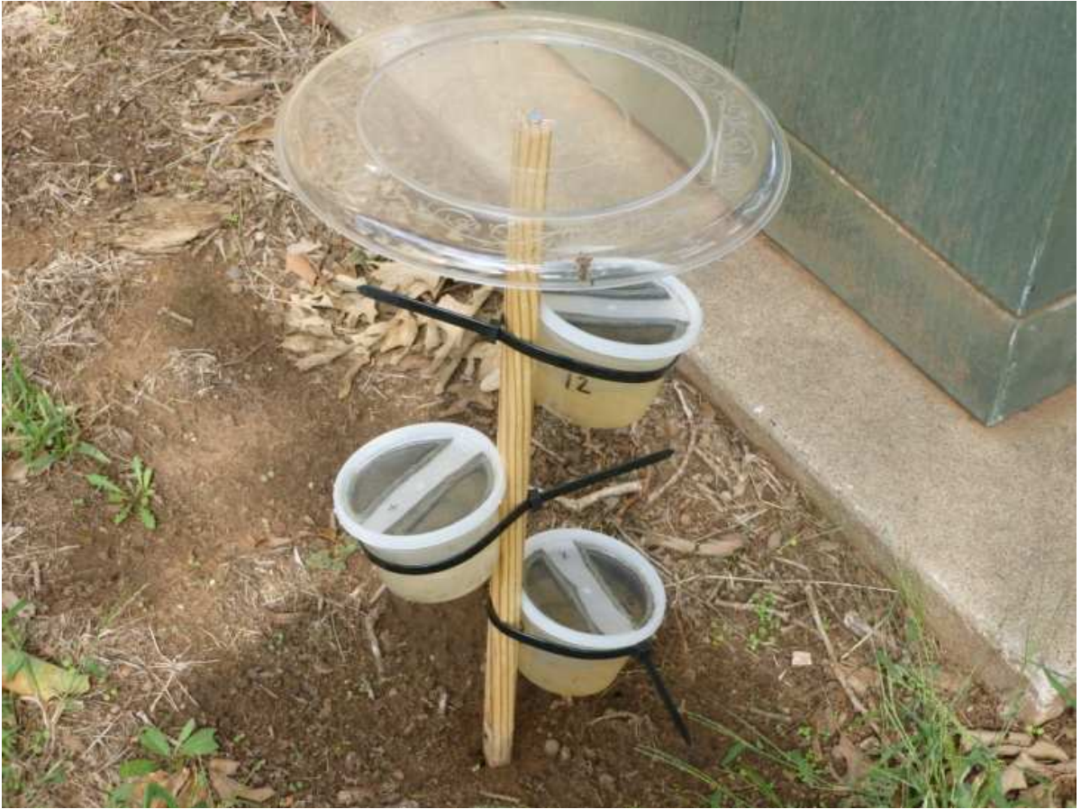
Figure 1. Container and stake design used during the field season. Each stake held three containers and two stakes were placed per site during the Urban Heat Island experiment.
