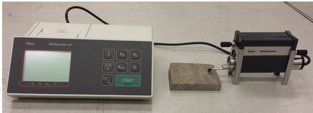
Figure 6.2 Perthometer set up for measuring limestone aggregate sample.
