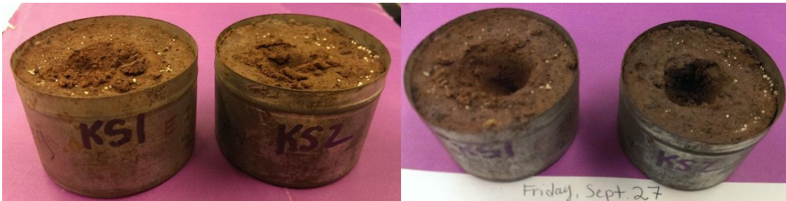
Figure 7. Samples KS1 and KS2 stored indoors (not exposed to direct light) on the left represents Day 1 (one hour) of soil extraction prior to testing, and on the right is the final day (96 hours) of extraction, prior to testing.
