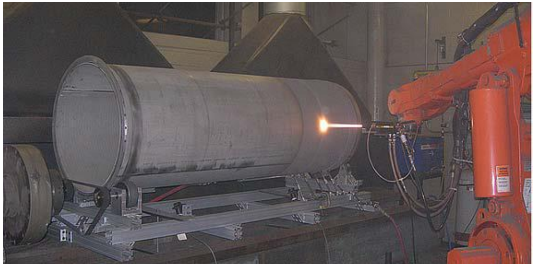
Fig.1.5 High-velocity oxy-fuel (HVOF) coating of SAM 1651 on half-scale spent nuclear fuel prototypical waste package [55].
