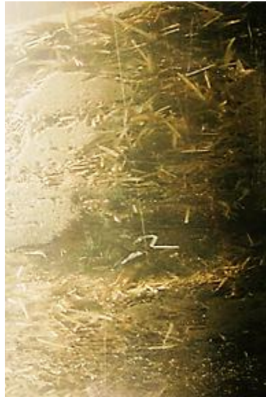
Fig. 3.7. Segregation of bed materials at 5% level of switchgrass in the mixture
