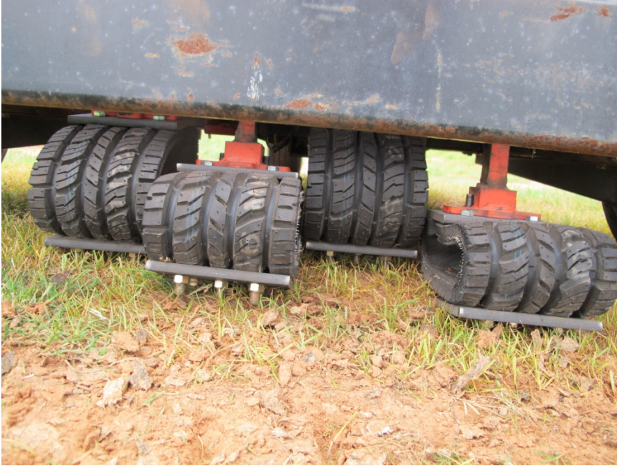
Figure 1c. Front view of feet of Cady Traffic Simulator.
