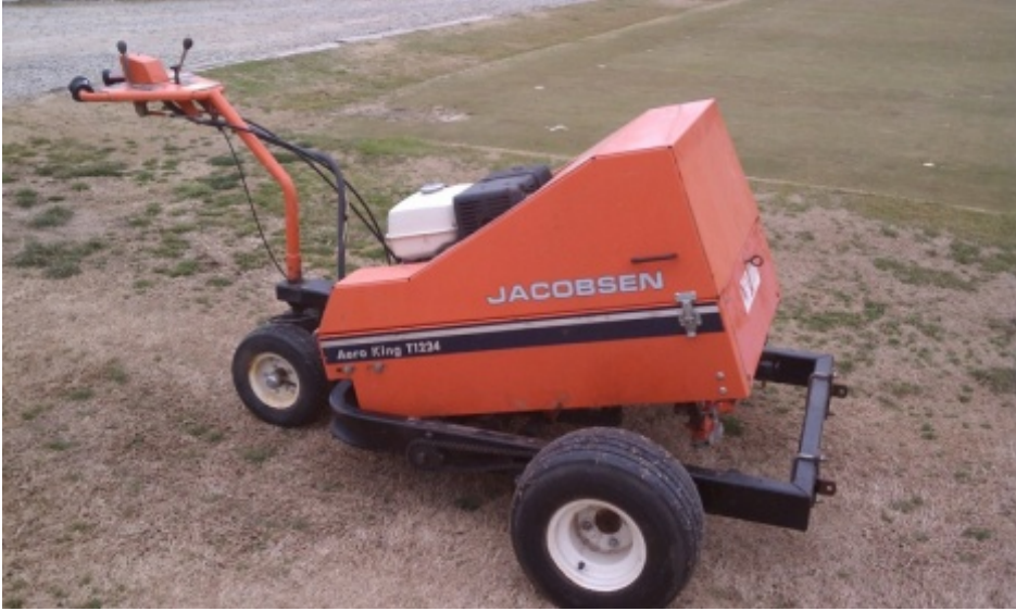
Figure 1a. Jacobsen T-1224 converted to Cady Traffic Simulator.
