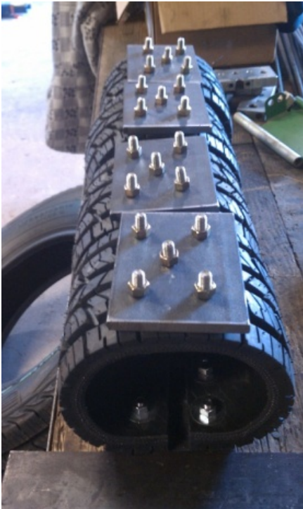
Figure 1b. Feet of the Cady Traffic Simulator.
