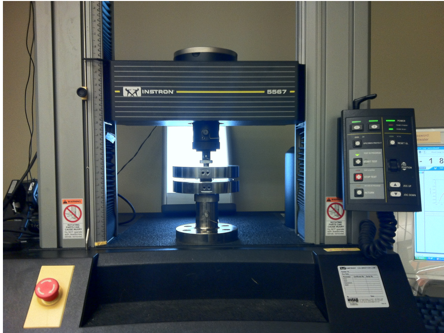
Figure II.2: Instron machine used for compression
