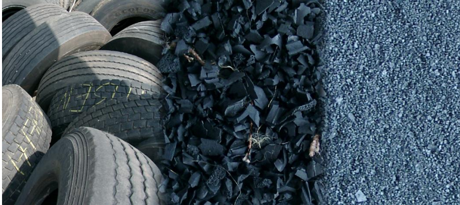
Figure I.1: Processing of crumb-rubber
