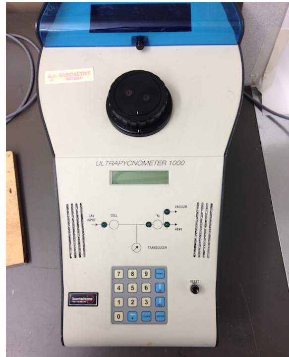
Figure II.4: Ultrapycnometer used to measure solid density
