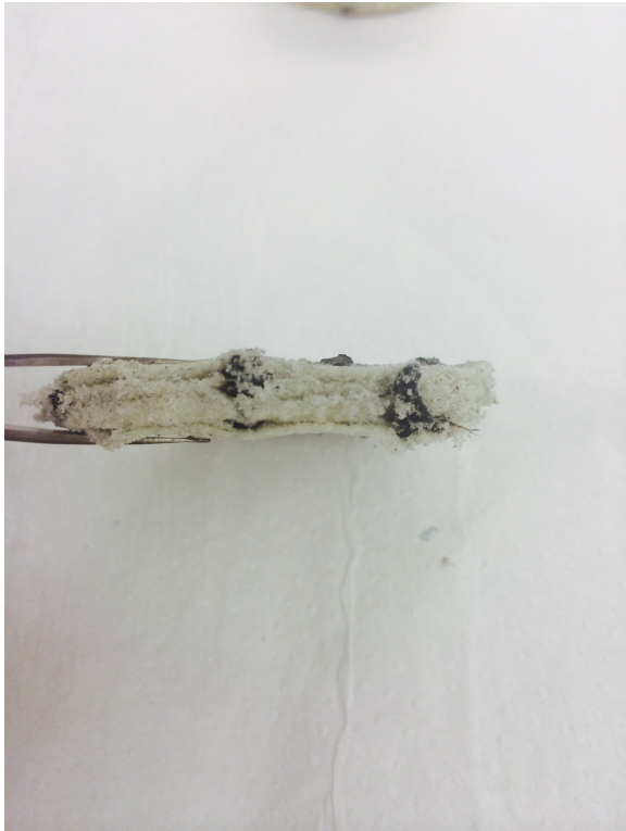
Figure III.18: Layered Crushing of Reinforced Foam
