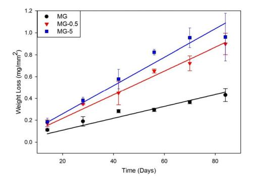
Figure 6-3. Weight loss of mild steel coupons in Miraclegro (MG) soils with various sodium chloride content.
