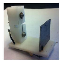
Figure 6-4. Zinc wire and mild steel coupon installed on holder for galvanic corrosion test.
