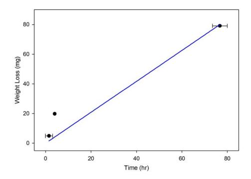
**Figure 6-5.** Weight loss of zinc wires due to galvanic corrosion in miraclegro soil containing 5% sodium chloride by weight (MG-5).
