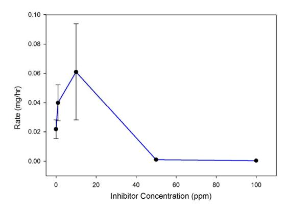
Figure 5-6. Iron wire corrosion rate in sodium chloride 0.5% solution in presence of calcium gluconate as inhibitor
