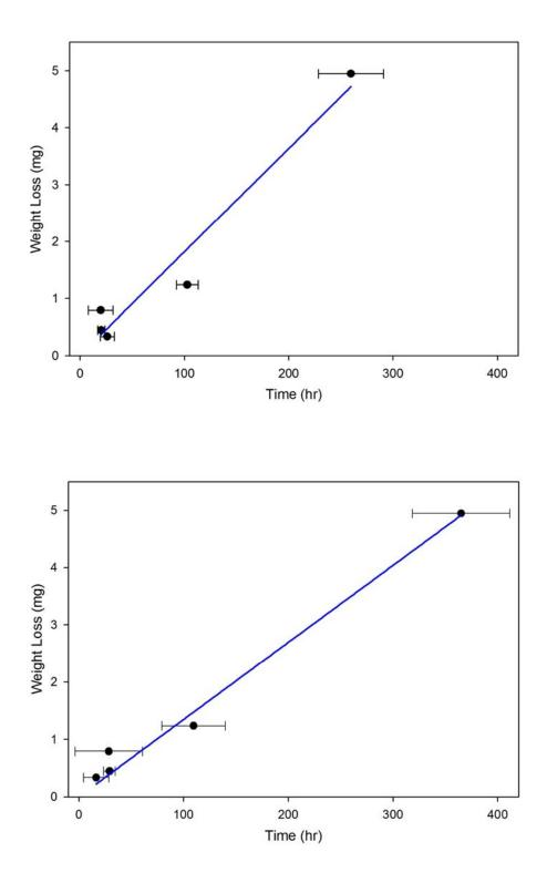
Figure 5-3. Weight loss of iron wires in sodium chloride solutions. (top) NaCl 0.5%, (bottom) NaCl 5%
