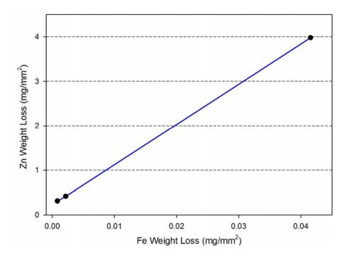
**Figure 6-6.** Galvanic corrosion of zinc wires and expected corrosion of mild steel coupons in miraclegro soil containing 5% sodium chloride by weight (MG-5)
