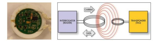
**Figure 6-7.** (left) Passive wireless corrosion sensor (right) Passive radio frequency identification (RFID) system
