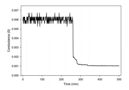
**Figure 5-2.** Wire conductance change with time for iron wire (r =0.065 mm) in sodium chloride 5% solution.
