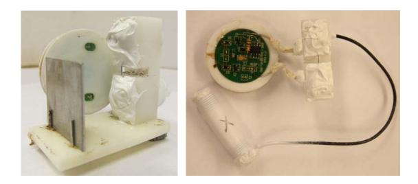
Figure 6-8. Sensor system for zinc galvanic corrosion in miraclegro soil containing 5% sodium chloride by weight (MG-5).
