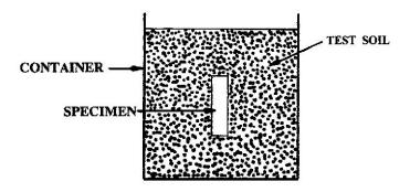
Figure 6-1. Apparatus for corrosion test in soil. (Figure adapted from Ref [126])
