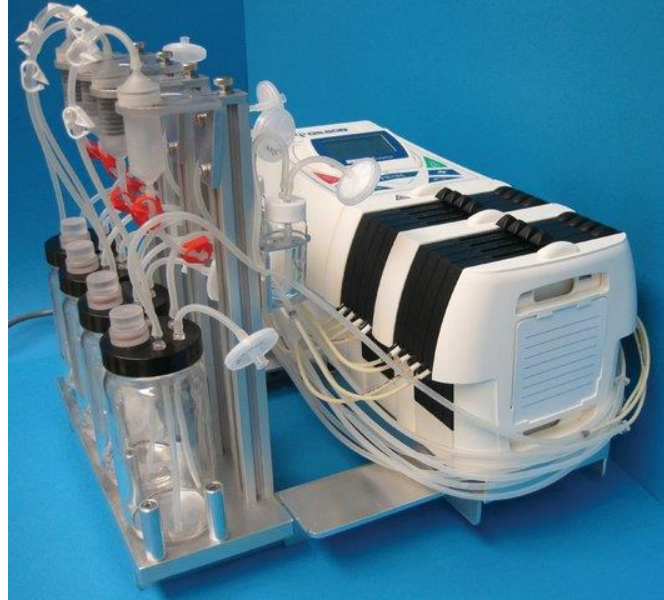
Figure 2.8 Perfusion bioreactor system with peristaltic pump from 3D Biotek LLC, North Brunswick, NJ.
