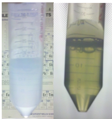
Figure 2: The Tyndall Effect Observed as the Lead Molybdate Solution Shown as a White Suspension (left), as it is Held up to a Light the Solution Turns from White to Yellow (right)
