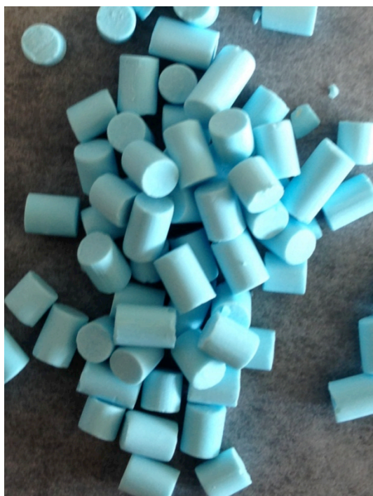
Figure 44: The Supported \text{CaWO}_4 after Treatment of Excess \text{Cu}^{2+}
