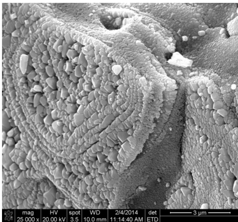
Figure 16: SEM Micrograph of the Starting Bulk-MoO 3 (top) and at Capacity (bottom)
