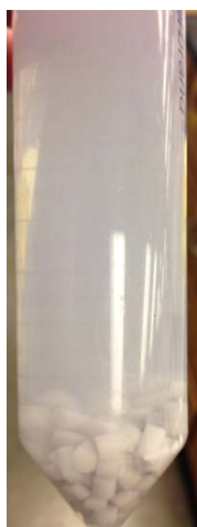
Figure 13: Formation of a PbMoO 4 Precipitate after Only 15 Minutes in the Kinetic Study
