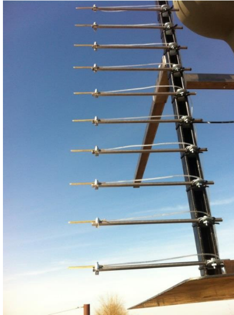
Figure 27-Full-Scale Test #1 Pitot-Rake Arrangement and Pitot Mounting
