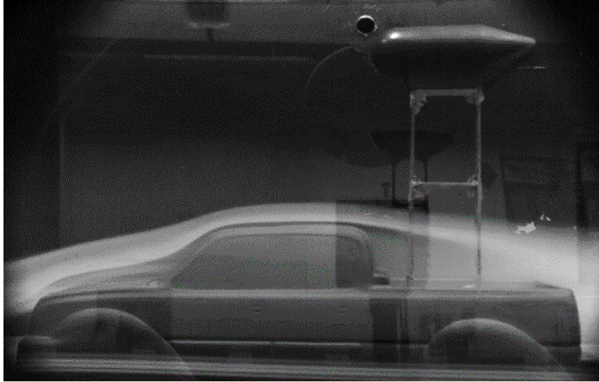
Figure 52-Flow Visualization With Dyno with Reynolds Number of 1.5 \times 10^6 (60mph)
