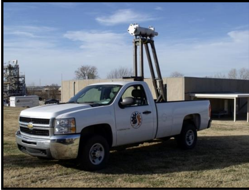
Figure 8-Mobile Dyno Installed in Test Vehicle (McGovney, 2010)
