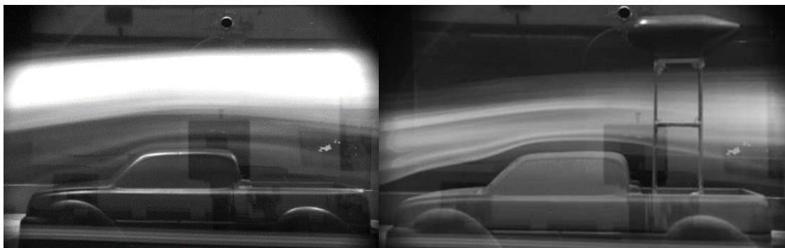
Figure 91-Flow Visualization With and Without Dyno with Reynolds Number of 4.9 \times 10^5 (20mph)
