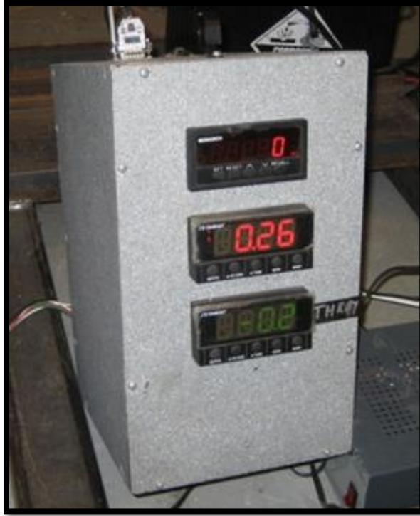
Figure 9-Mobile Dyno Display and Signal Conditioner Box (McGovney, 2010)
