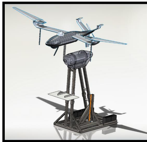
Figure 53-VTOL Aircraft Installed to Allow Dynamic Tests of Transition
