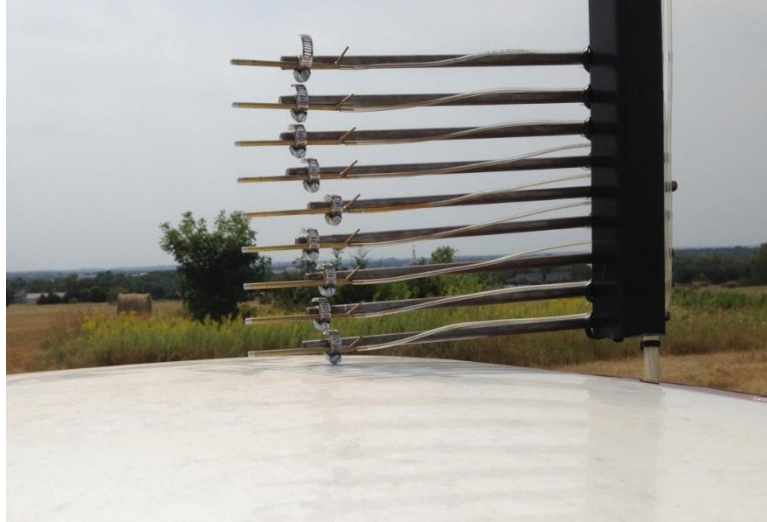
Figure 36-Pitot-Probe mounting for Full-Scale Test #2
