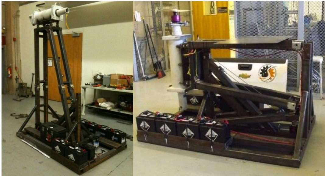
Figure 7-Mobile Dyno in Collapsed and Test Position (McGovney, 2010)
