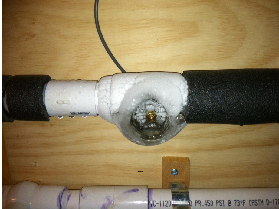
Figure 2.28: Gem flow meter during heat extraction test
