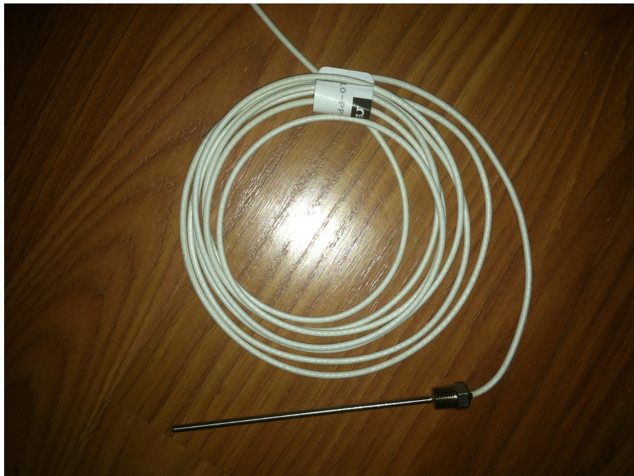
Figure 2.23: In-pipe thermistor used to measure circulating fluid inlet and outlet temperature
