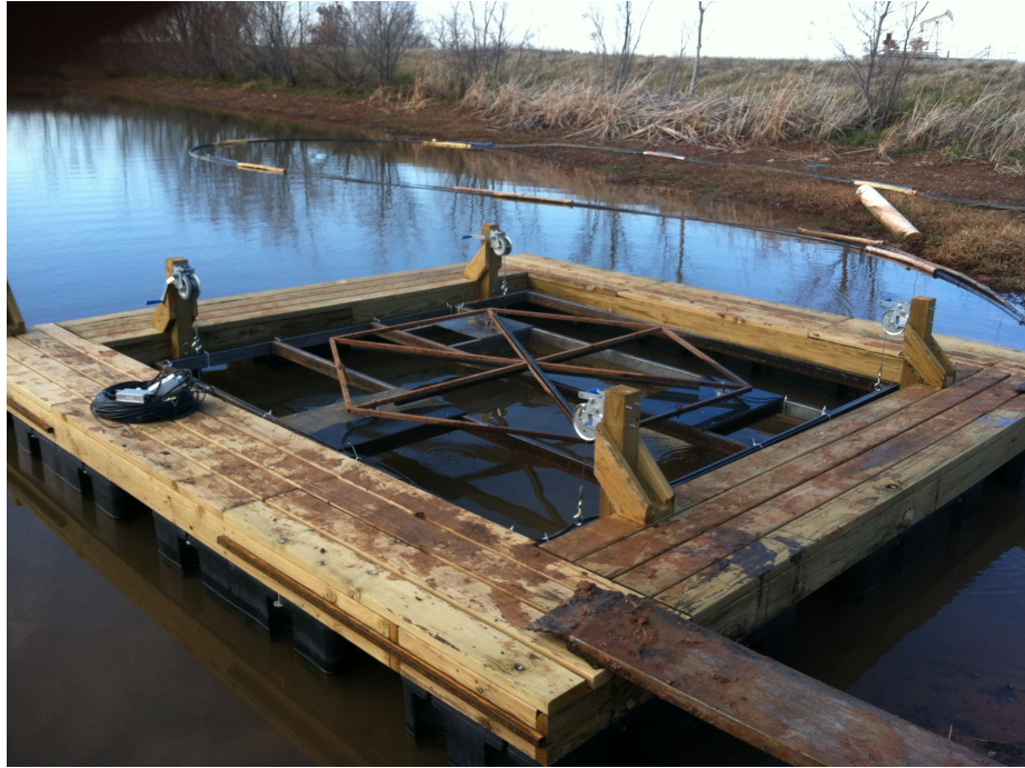
Figure 2.15: Heat extraction experiment support platform and load cell frame
