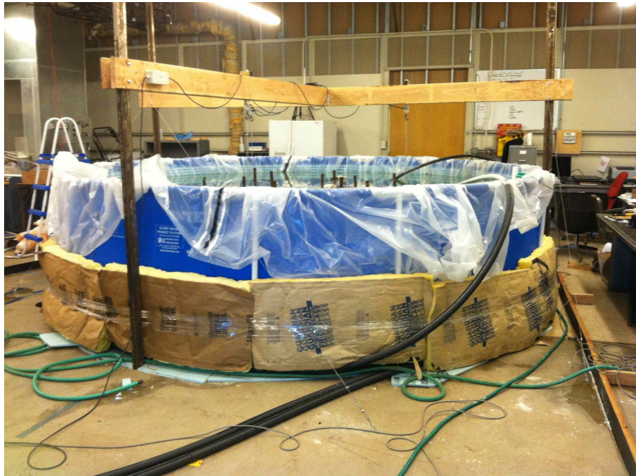
Figure 2.18: Experimental setup used for indoor heat exchanger tests
