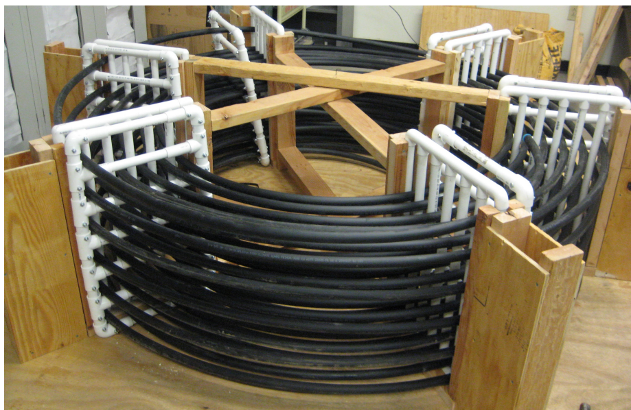
Figure 1.4: Photo of spiral-helical heat exchanger. Reprinted, by permission, from Hansen (2011)
