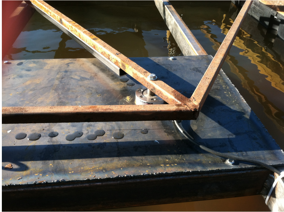
Figure 2.13: Submersible load cell used to measure buoyancy force
