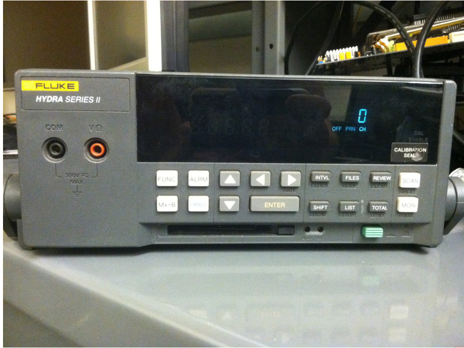
Figure 2.27: Fluke data logger used to measure and record flow and temperature measurements
