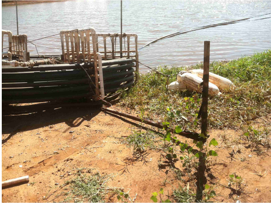
Figure 2.7: L-arm at a distance of 4 ft. (1.2 m) away from coil used for measuring local pond temperature
