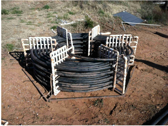
(a) Spiral-helical surface water heat exchanger prepared for testing.
