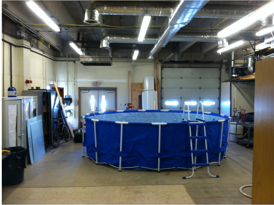
Figure 2.17: Pool used for testing spiral-helical SWHE in laboratory facility
