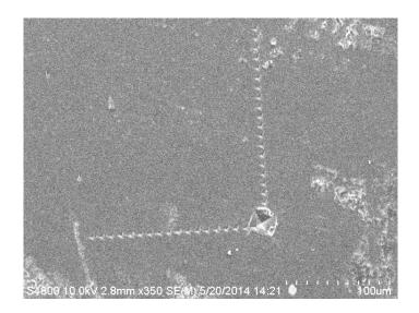
Figure III.19: SEM: Nanoindents around vickers Indent
