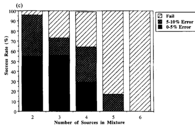
Figure 11 The fail rates for the mixing experiments regarding different number of sources - comparing fingerprinting method and the actual mixing proportion (Lees, 1997).
