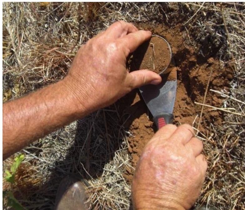
Figure 15 Rangeland surface soil sampling using a soil ring.
