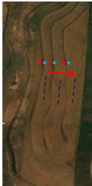
Figure 48 Aerial Photograph of Transect 11 (Google Earth, 2012). Red dots were the upslope terrace bank; blue dots were the downslope terrace bank; blue dash lines were where soil samples were collected; red line shows the estimated flow direction.
