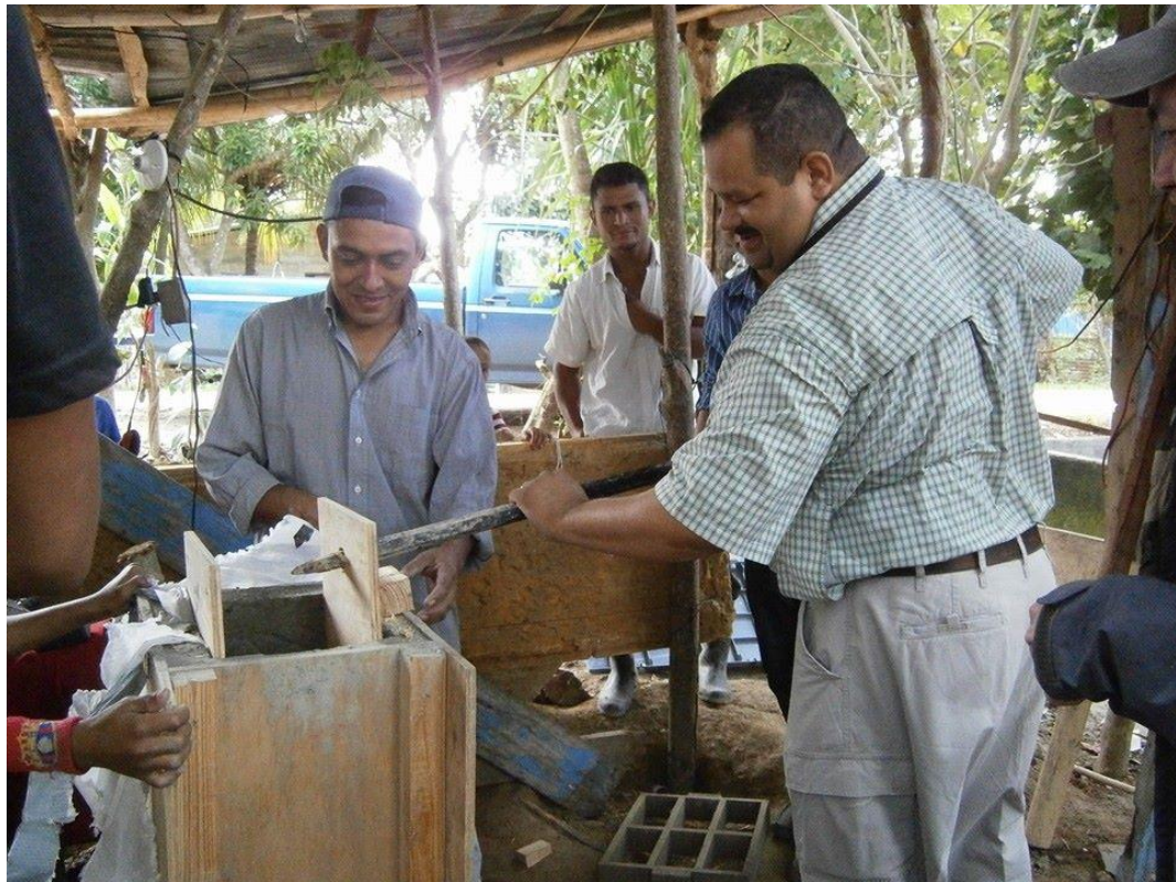
Figure 19: Leveraging Inner Mold Panel for Removal
