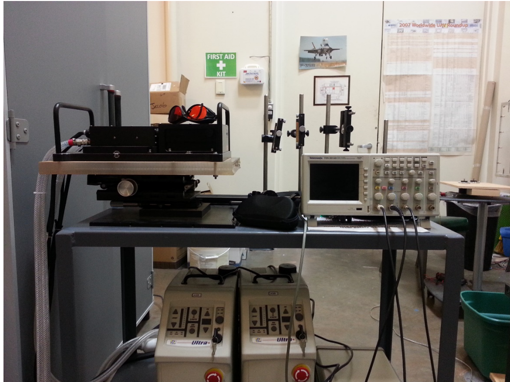
Figure 27 Laser setup for PIV.
