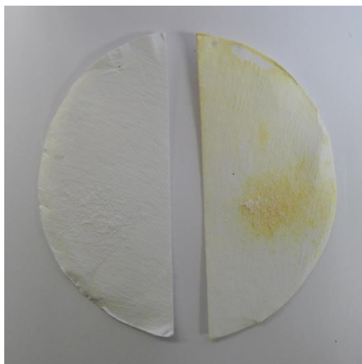
Figure V-3. (Left) Hydrochloric and (right) sulfuric acid coatings following a surface contact test with HMTD.
