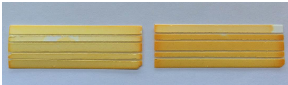
Figure V-6. Coatings exposed to peroxide after aging for (left) one day and (right) two weeks. The strip was made in accordance with the described layout in Section B.3 of this Chapter. The increased orange content of the older coating can be clearly seen.
