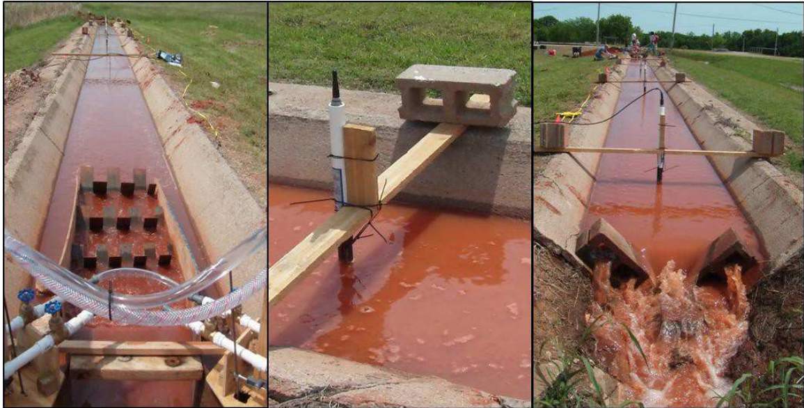
Figure 6. Testing setup at the upstream end of the turbidity reduction system. Sediment introduction took place at the beginning of the channel into a mixing chamber, passed through a flow straightener into a forebay, then through the dosing and mixing system, and into the setting channel.
