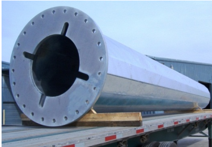
Figure 1.4. Galvanized pole about to be shipped
