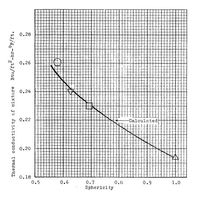
Figure IV-2. Comparison of calculated and measured conductivities of mixtures with 16 volume percentage aluminum particles of various chapes in silicone 'Silastic' rubber. The curve was calculated from equation III-25 with  $n = 3/\psi$ ;  $\Delta$  spheres; [] cylinders, 5 X 1 mm diameter; () cylinders, 2.7 X 0.27 mm diameter;  $\nabla$  parallelepipeds, 1.6 X 1.6 X 0.4 mm
