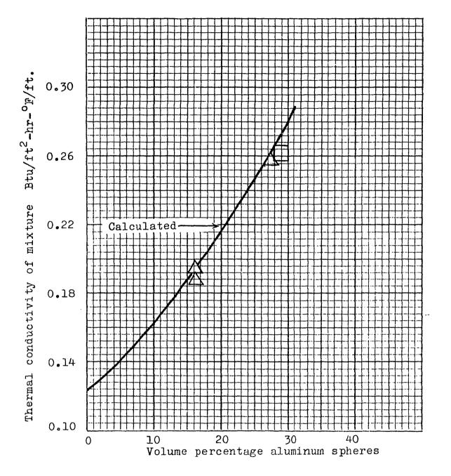
Figure IV-1. Comparison of calculated and measured conductivities of mixtures of aluminum spheres in silicone 'Silastic' rubber. The curve was calculated from equation III-25 with n = 3;  $\Delta 1.2$  mm diameter spheres;  $\bigcirc 0.012$  mm diameter spheres
