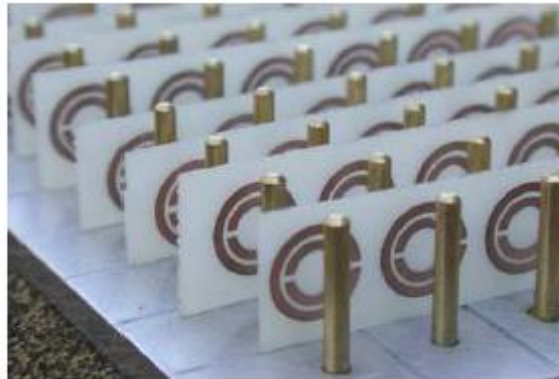
Figure 1-5 Double-negative material comprised of metal wires and SRRs to realize the negative refractive index metamaterials [31,35].
