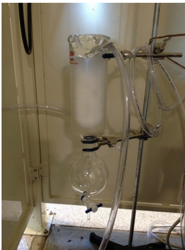
Figure 3.39 Measurement of solvent loss using a dry ice condenser trap
