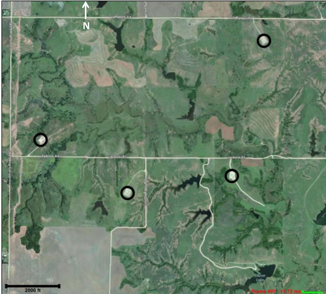
Figure 5: Well surface locations represented by black circles are displayed over a live Bing map using Transform software. Drilling pads, still visible from the live map, confirm that the well locations are in the correct place from a map view perspective.
