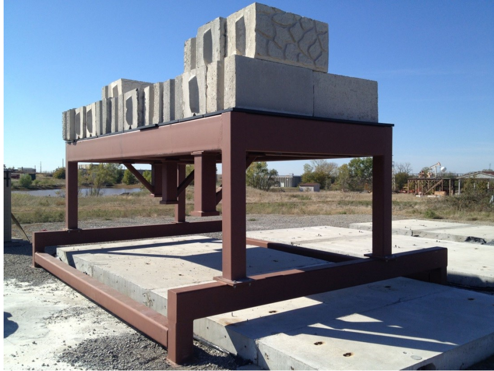
Figure 47 Final test frame assembled and ready for testing for Pavement III
