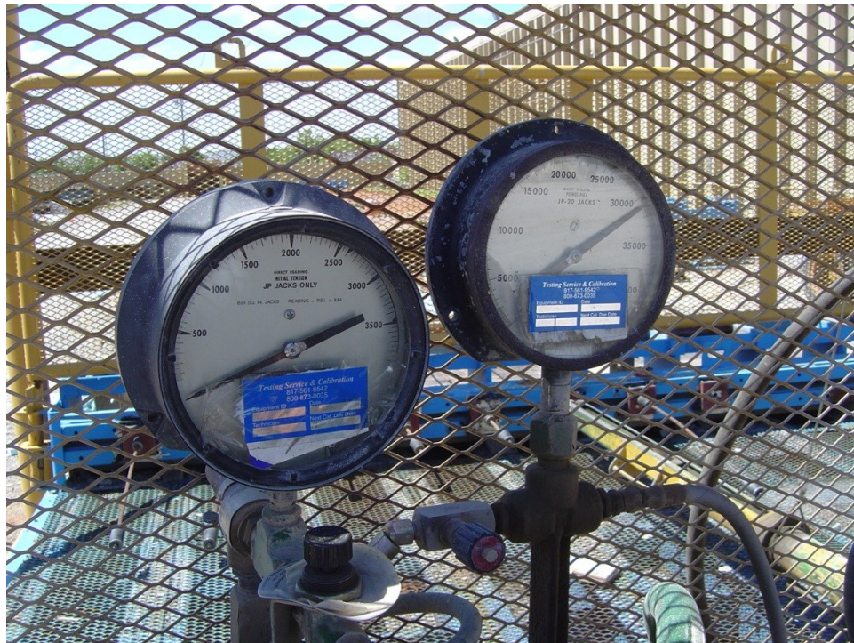
Figure 19 Pressure indicators used to measure tension force in pretensioned strands
