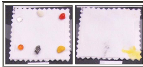
Figure B.7: Formulation PA2 treated fabric (a) with stains (b) after wiping stains
