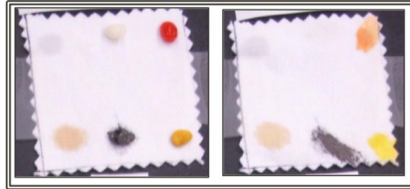
Figure B.6: Untreated Interlock fabric (a) with stains (b) after wiping stains
