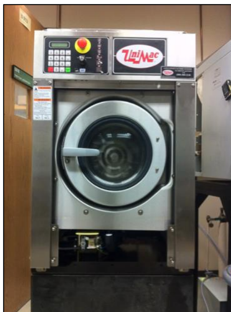
Figure B.14: Unimac exhaust dyeing unit
