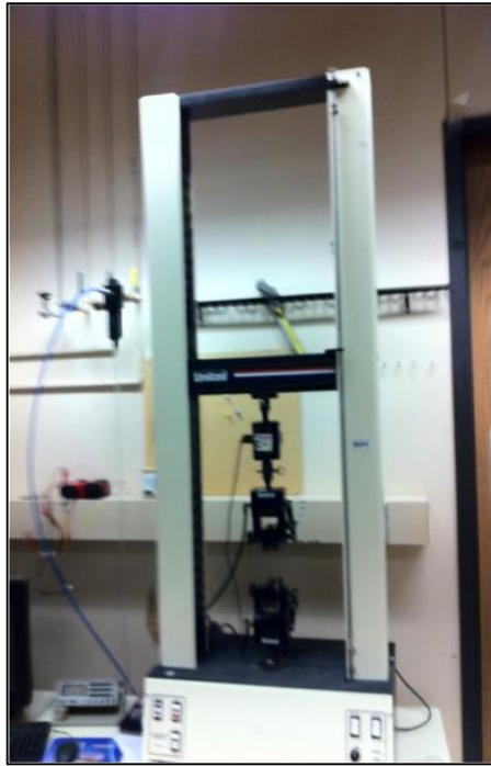
Figure B.4: SSTM tester according to ASTM D1708
