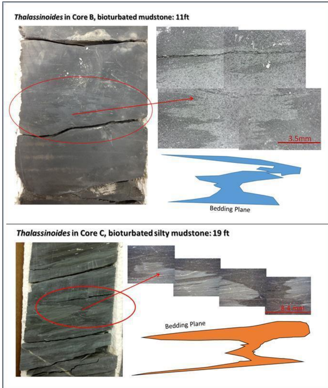
Figure 4.10. Examples of Thalassinoides in Core B and C, both examples are in Lower Woodford. The materials in vertical burrows are coarser grained than surrounding matrix, with occasionally pyritized framboid in them (Photos by Kimberly Hlava).
