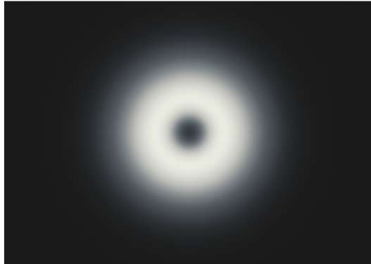
Figure 6.4: The model given by equation 6.1. The parameters used in the model are similar to the parameters used in figure 2.20. The control Rabi frequency is \Omega_{0c,12} = 20 MHz. The linewidth of the control laser is assumed to be \gamma_c = 1 MHz, the linewidth of the probe laser is set \gamma_p = 0.1 MHz, the number density is set to N = 5 \times 10^{10} \text{ cm}^{-3} , and the detuning of the control laser and the probe laser are set to \Delta_c = \Delta_p = 0 . Due to the spatial dependence of a \text{LG}_0^1 mode laser, the model predicts that the transmission of the probe matches the intensity profile of the \text{LG}_0^1 laser.
