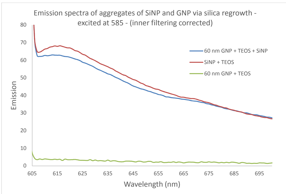
Figure 4.53. Emission spectra of aggregates of 60 nm GNP and previously synthesized QD-doped-SiNP via silica regrowth.
