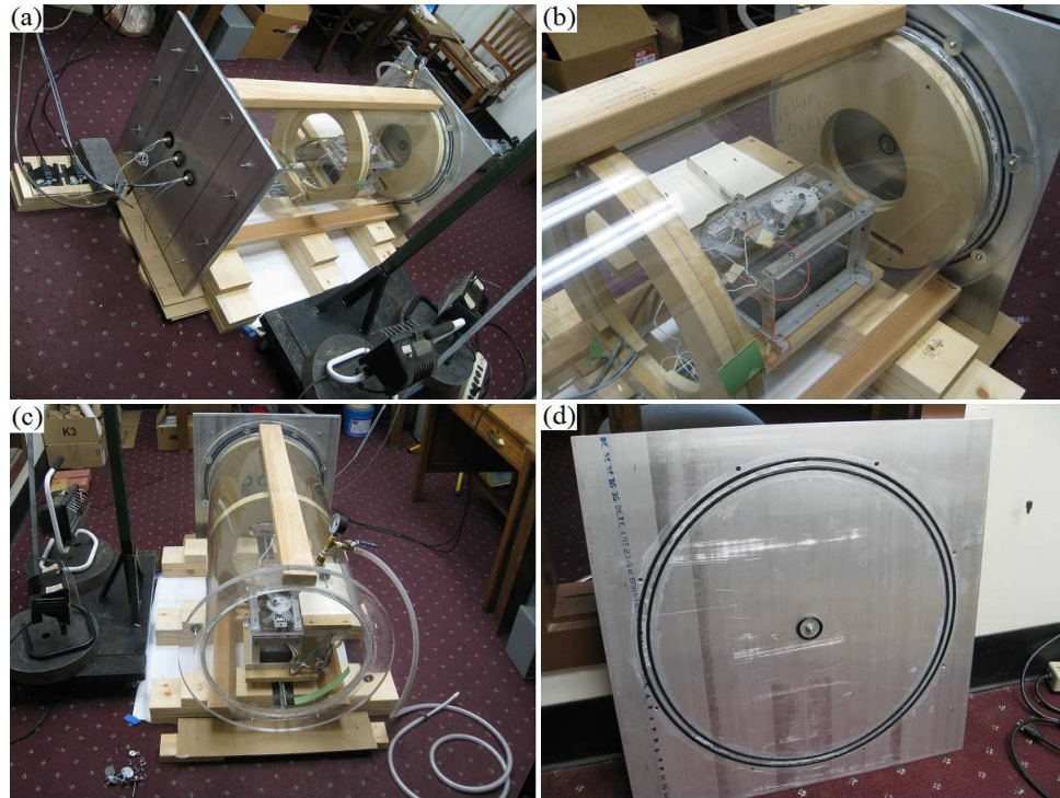
Figure 2.13: Vacuum chamber: (a) stationary cover end with electrical feedthrough for strain gage and motor cables, (b) flapping mechanism placed in the chamber, (c) access cover end, (d) aluminum cover with double O-rings.
