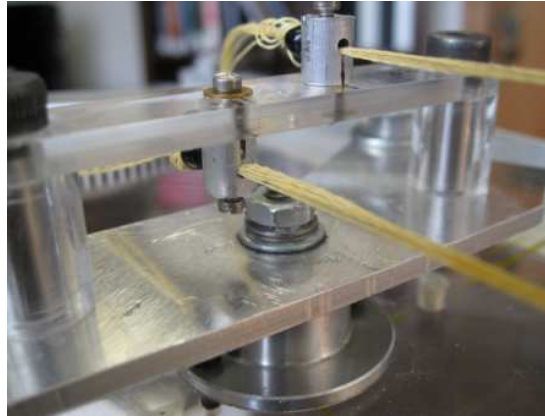
Figure A.7: Close-up view of cylindrical aluminum standoffs which connect the strings to the rocker link. Kevlar ™ strings are used for increased tensile strength.
