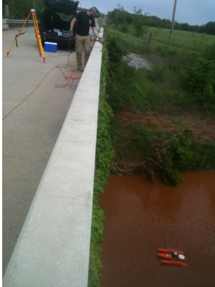
Figure 12: Discharge measurement using Acoustic Doppler Current Profiler (ADCP) at the Little River at 60 th site.
