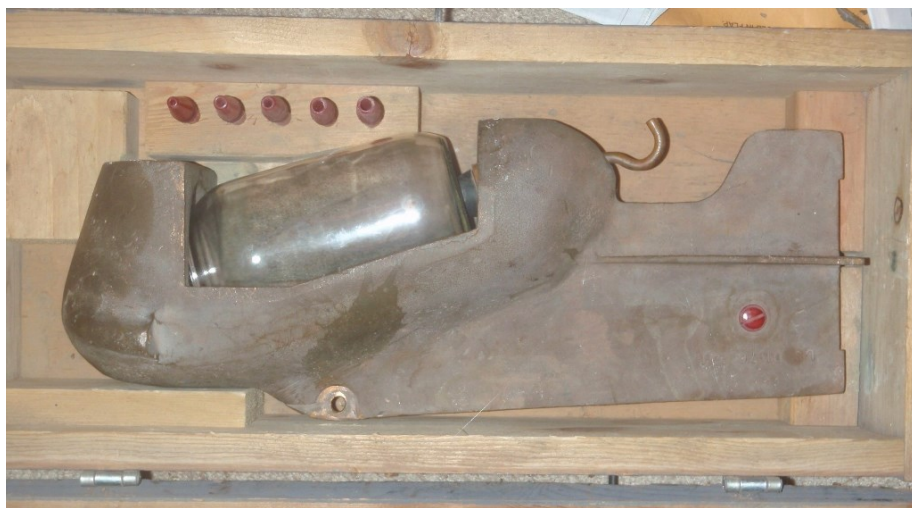
Figure 67: FISP DH-76 isokinetic depth integrated sampler.
