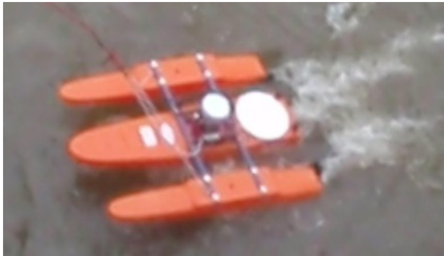
Figure 66: Teledyne RDI 600 kHz Workhorse Rio Grande OceanScience Riverboat with RTK GPS.
