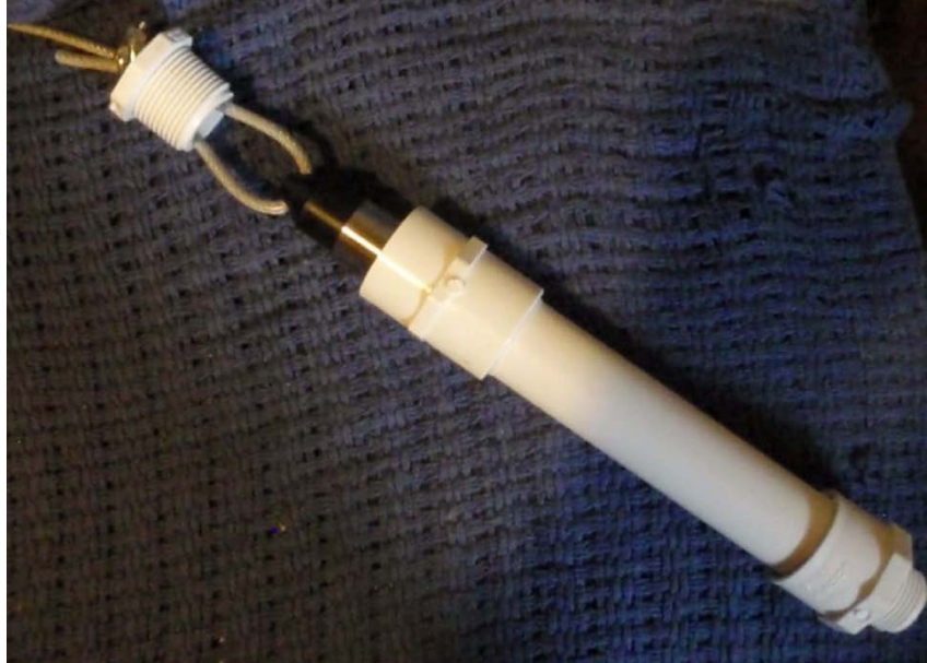
Figure 8: HOBOTM water level logger with PVC housing.
