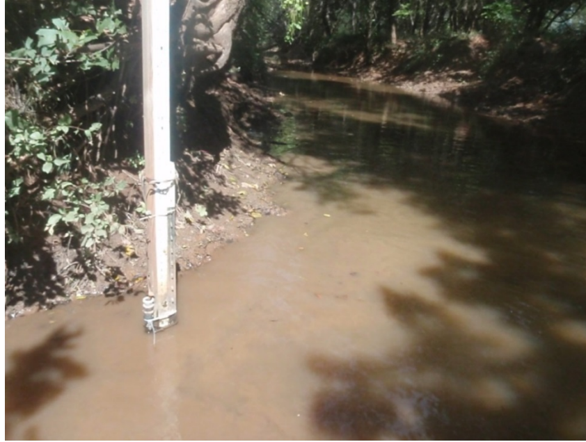
Figure A.3.2: Hog Creek at SE119th Ave site HOBOT installation.
