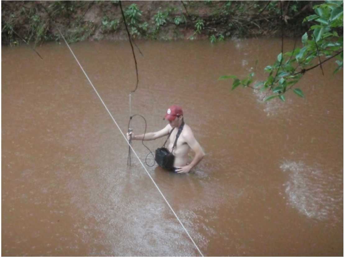
Figure 10: Discharge measurement using Marsh McBirney flow meter at the Little River at 60 th site.
