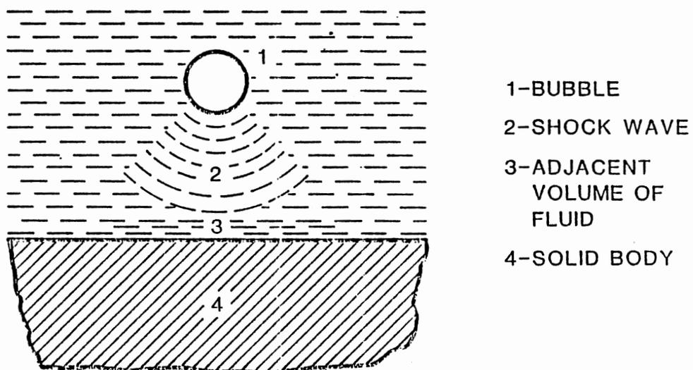
Figure 3. Collapse of cavitation bubbles [41]
