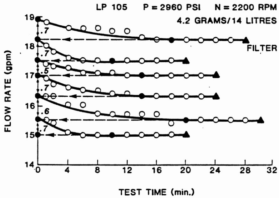
Figure 19. Pump flow degradation from multiple injections
