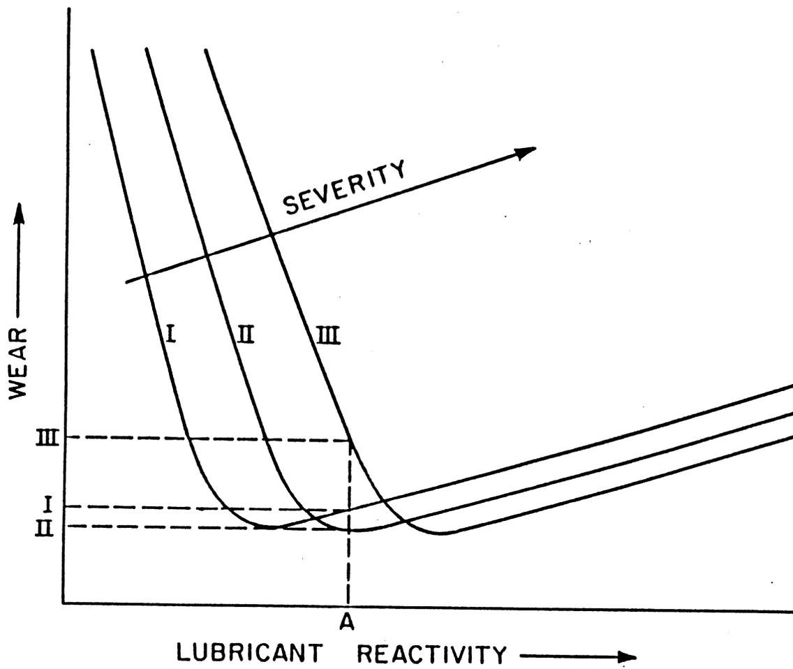
Figure 36. Schematic illustration of the severity of sliding on adhesive-chemical wear balance
