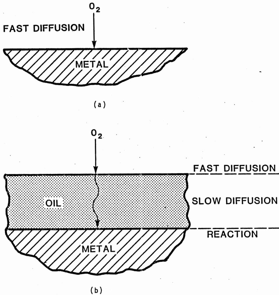
Figure 7. Effects of the surface film on oxygen diffusion:
