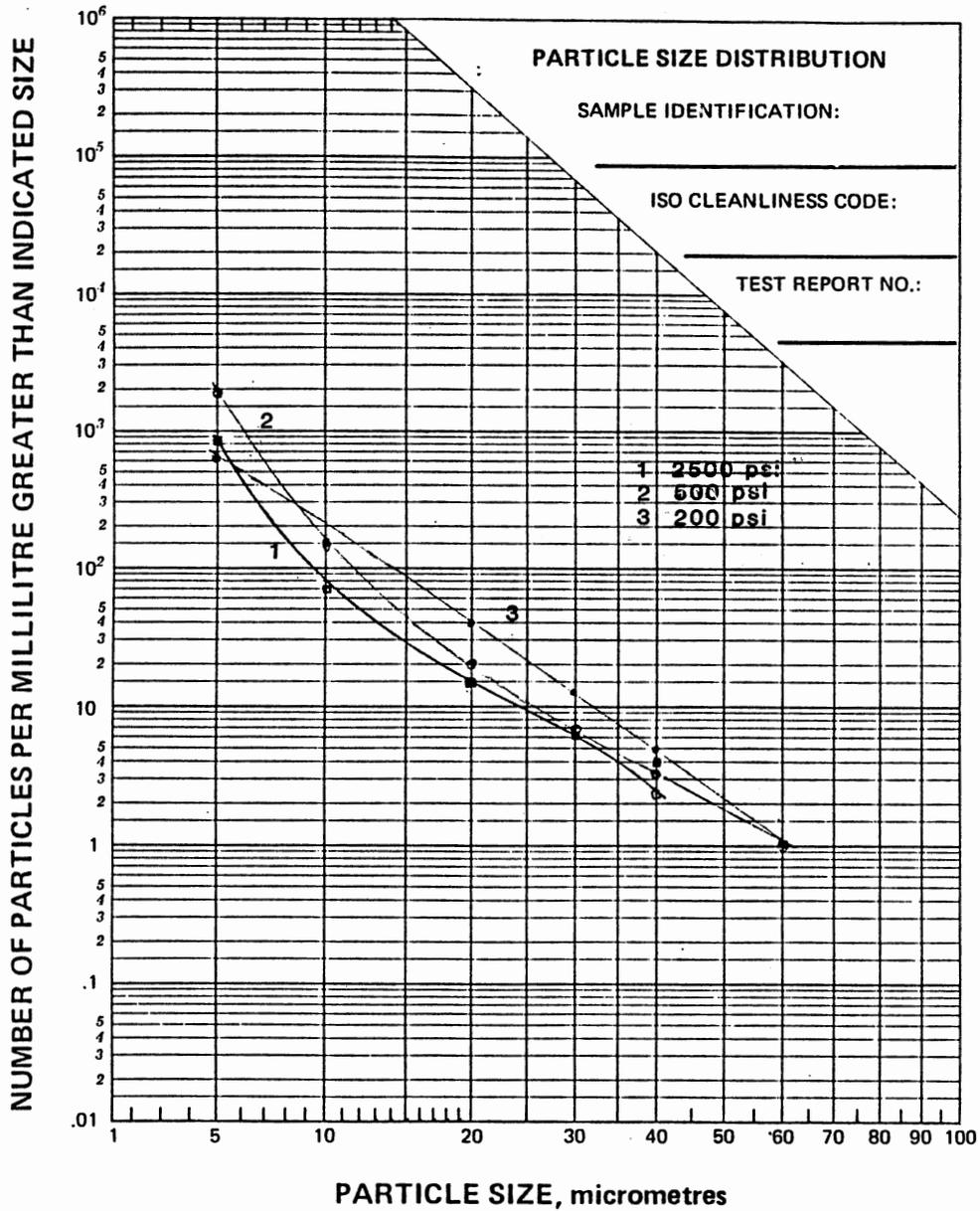
Figure 29. Particle size distribution obtained after six hours of testing. Adhesion wear - Pump 539
