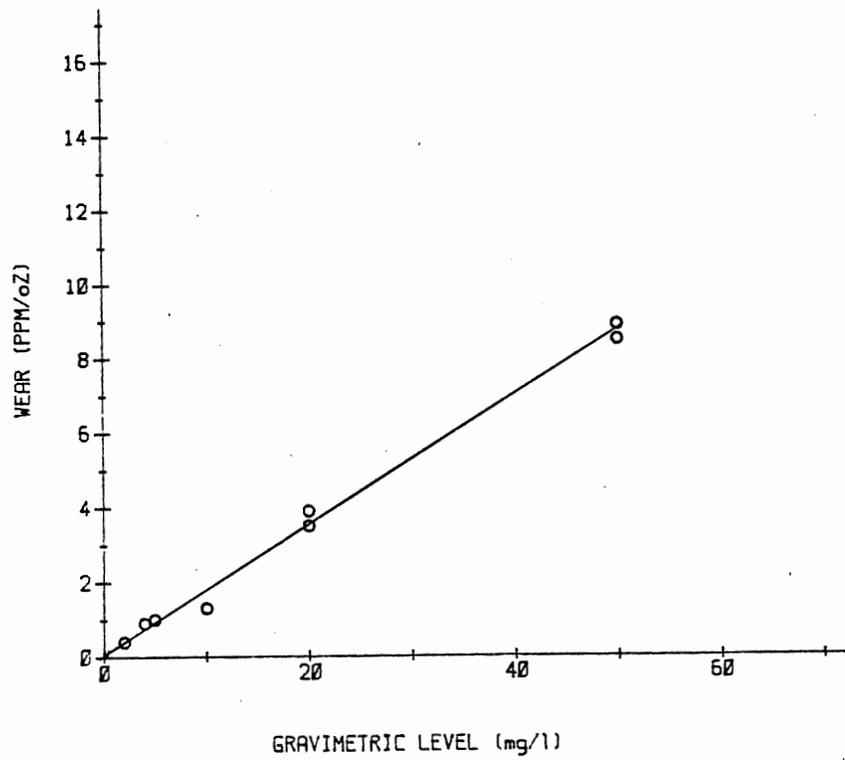
Figure 21. Sensitivity of wear analyzer readings
