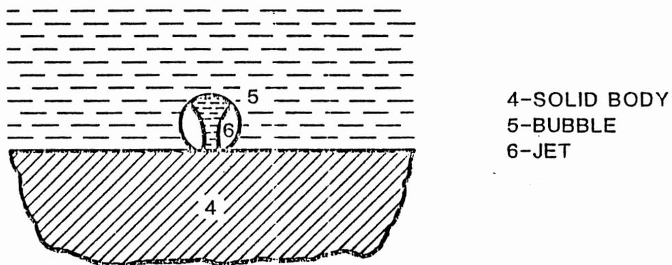
Figure 4. Collapse of cavitation bubbles [42]
