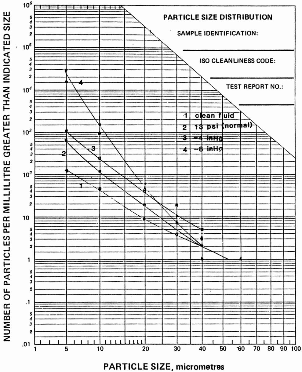
Figure 24. Particle size distribution obtained after six hours of testing. Cavitation wear - Pump 531
