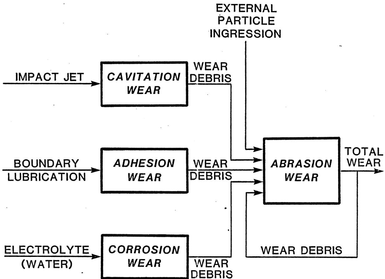
Figure 13. Synergistic view of pump wear process
