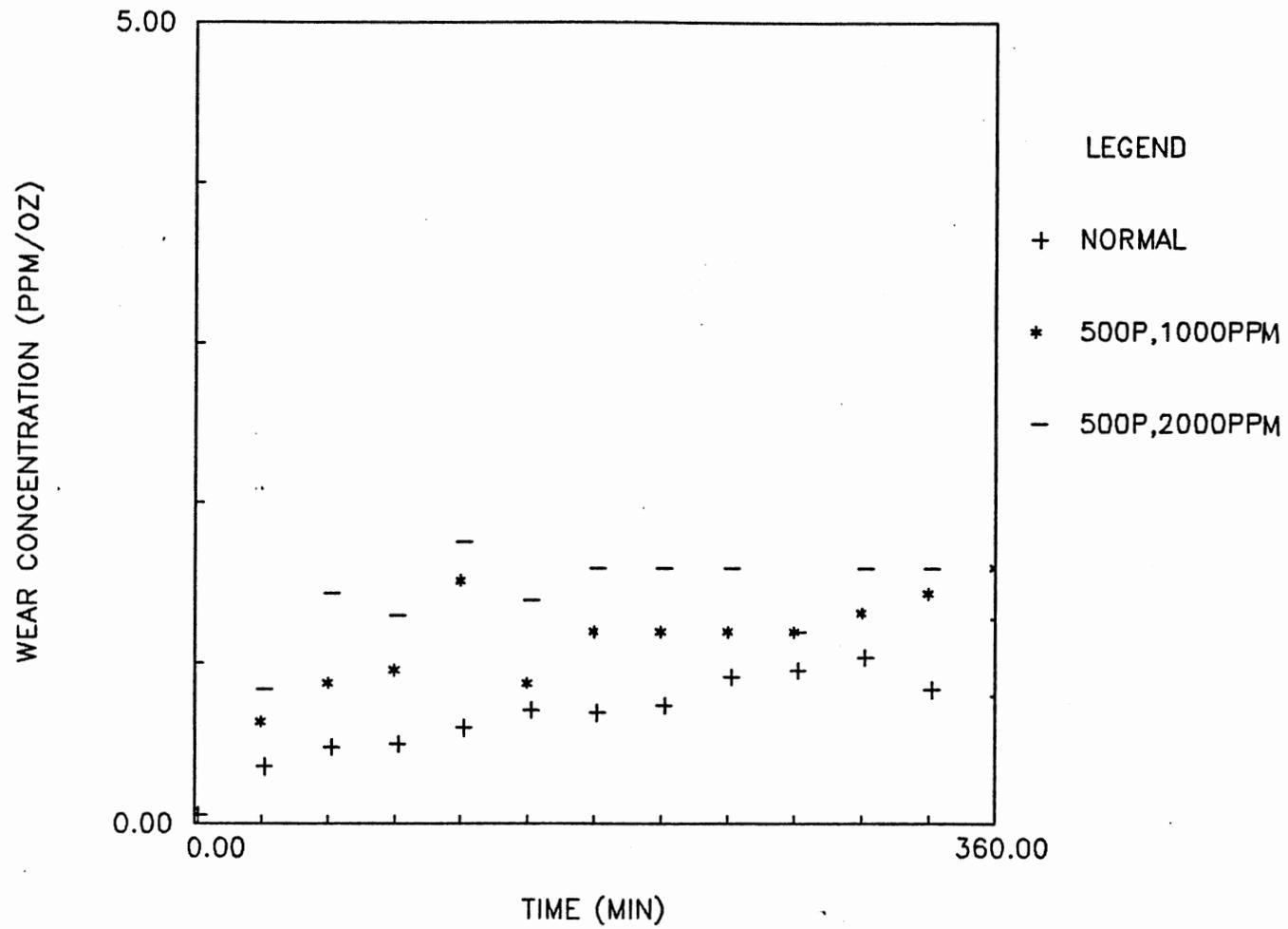
Figure 35. Magnetic wear debris generated under corrosion-adhesion conditions
