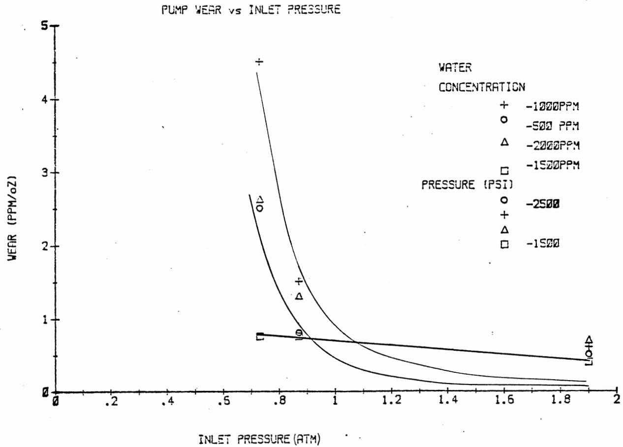
Figure 42. Wear concentration vs. Inlet pressure.
