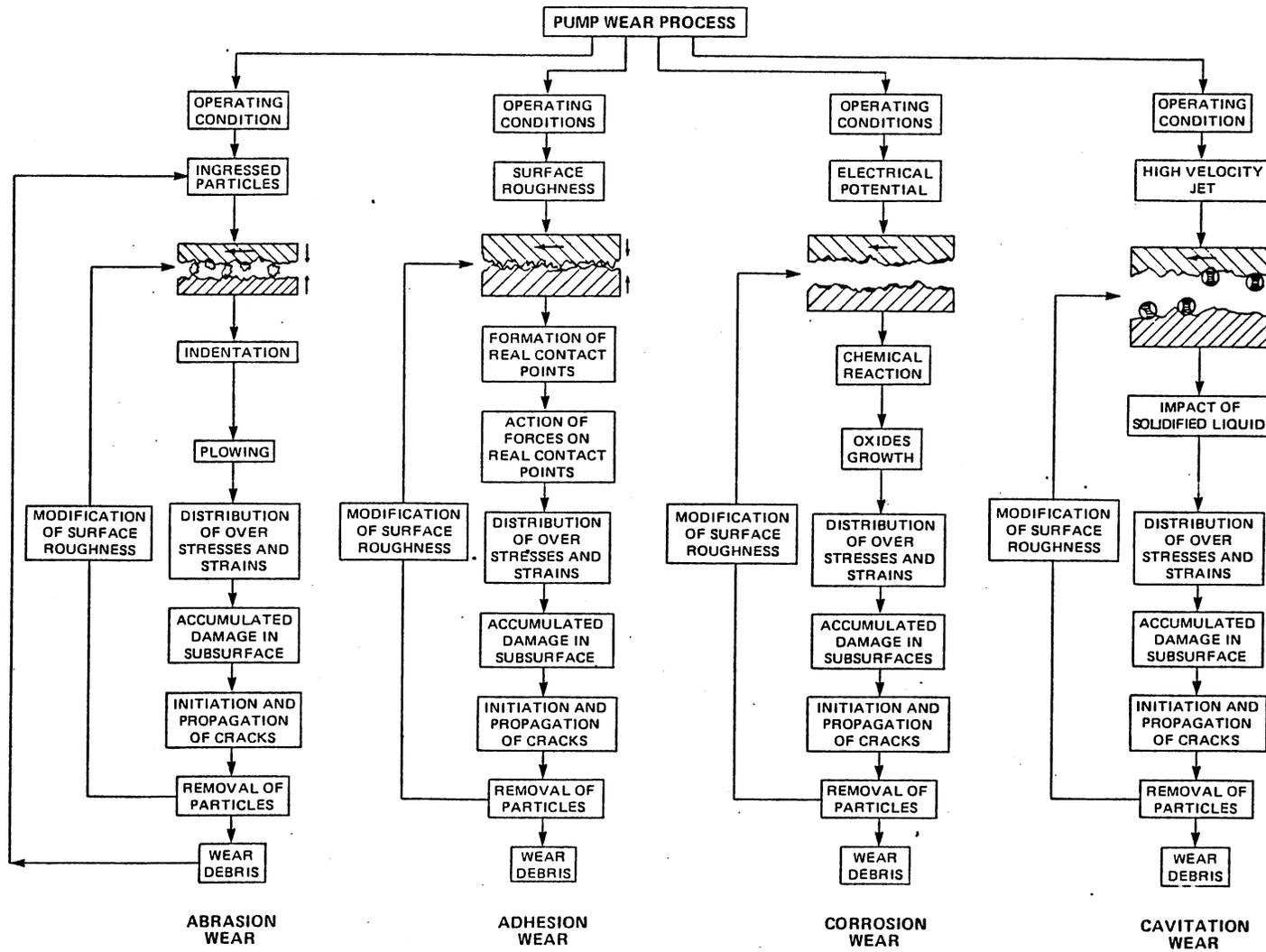
Figure 9. Breakdown of pump wear process
