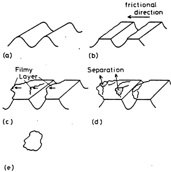
Figure 14. Wear particle generation under boundary lubricated conditions - forward plastic flow
