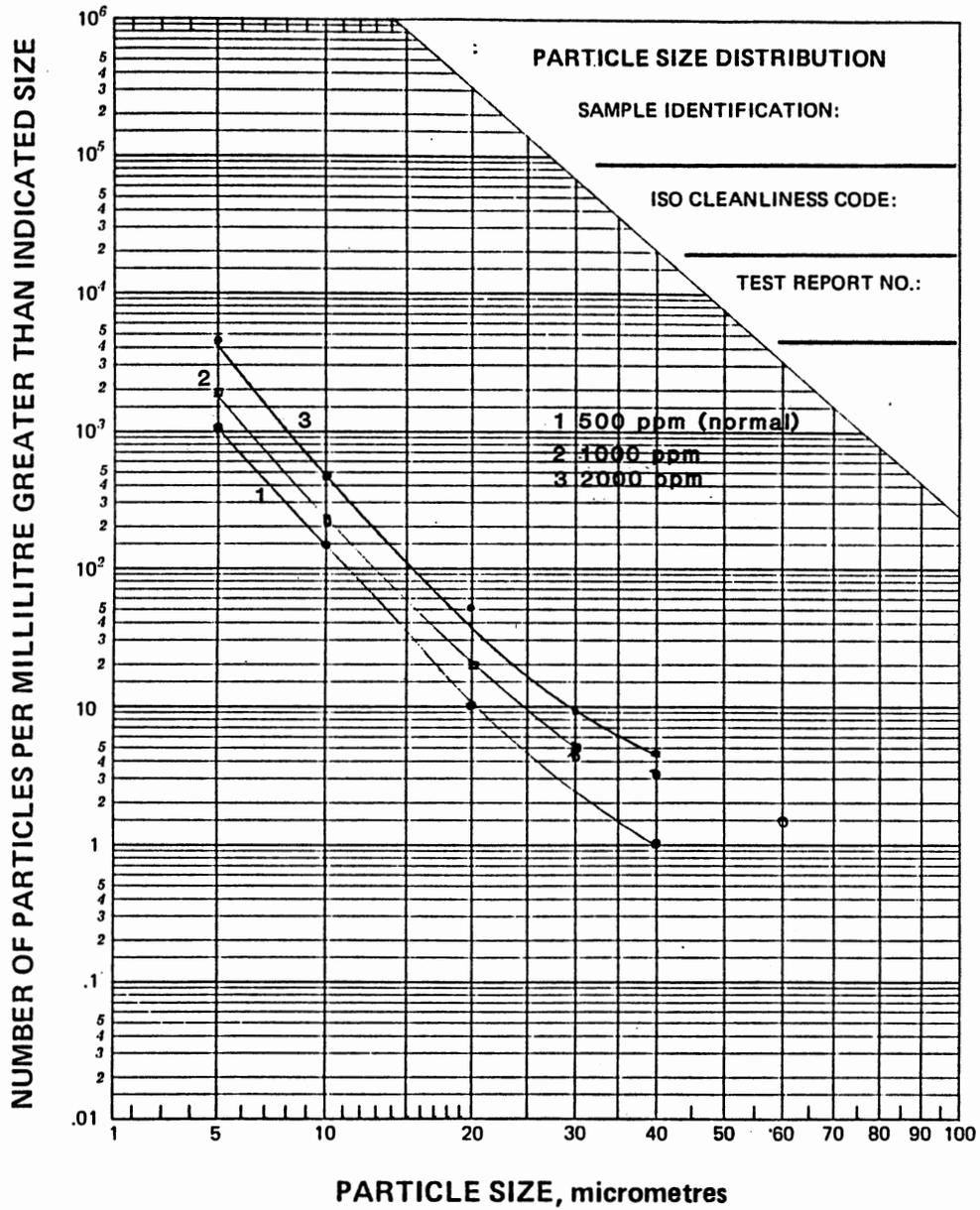
Figure 31. Particle size distribution obtained after six hours of testing. Corrosion wear - Pump 533
