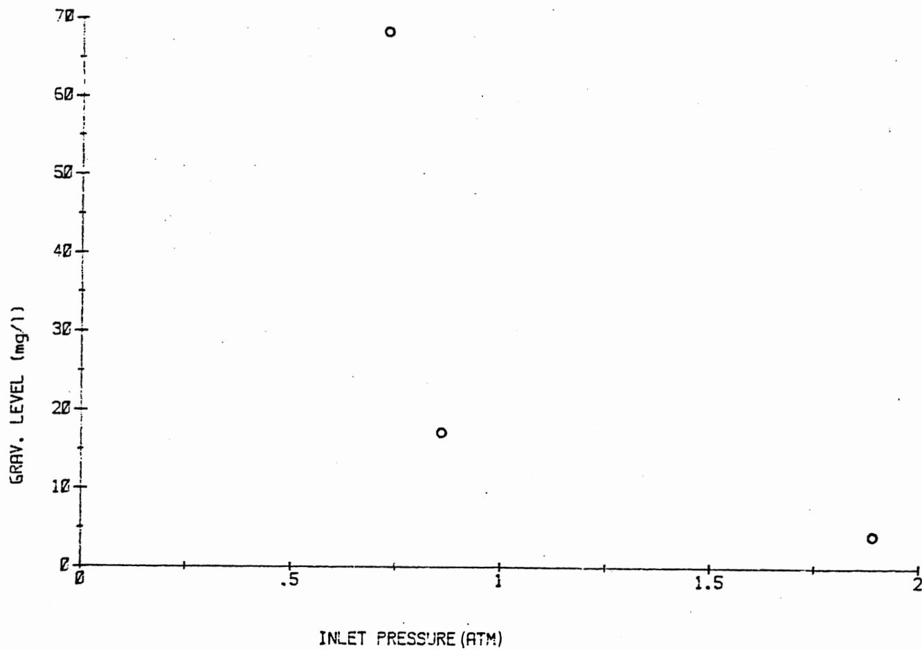
Figure 27. Fluid gravimetric levels - Cavitation wear - Pump 531
