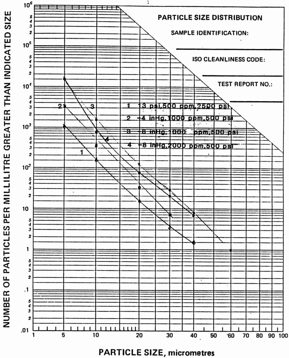
Figure 41. Particle size distribution obtained after six hours of testing. Cavitation-Corrosion-Adhesion wear - Pump 663
