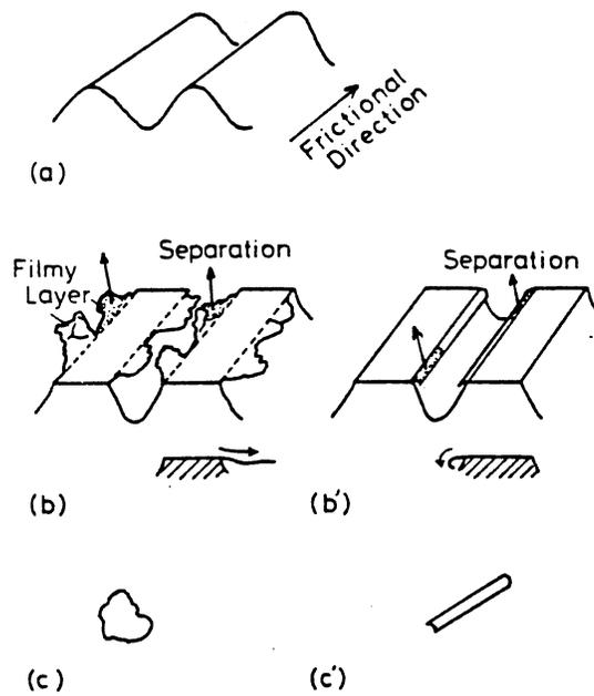
Figure 15. Wear particle generation under boundary lubricated conditions - side plastic flow
