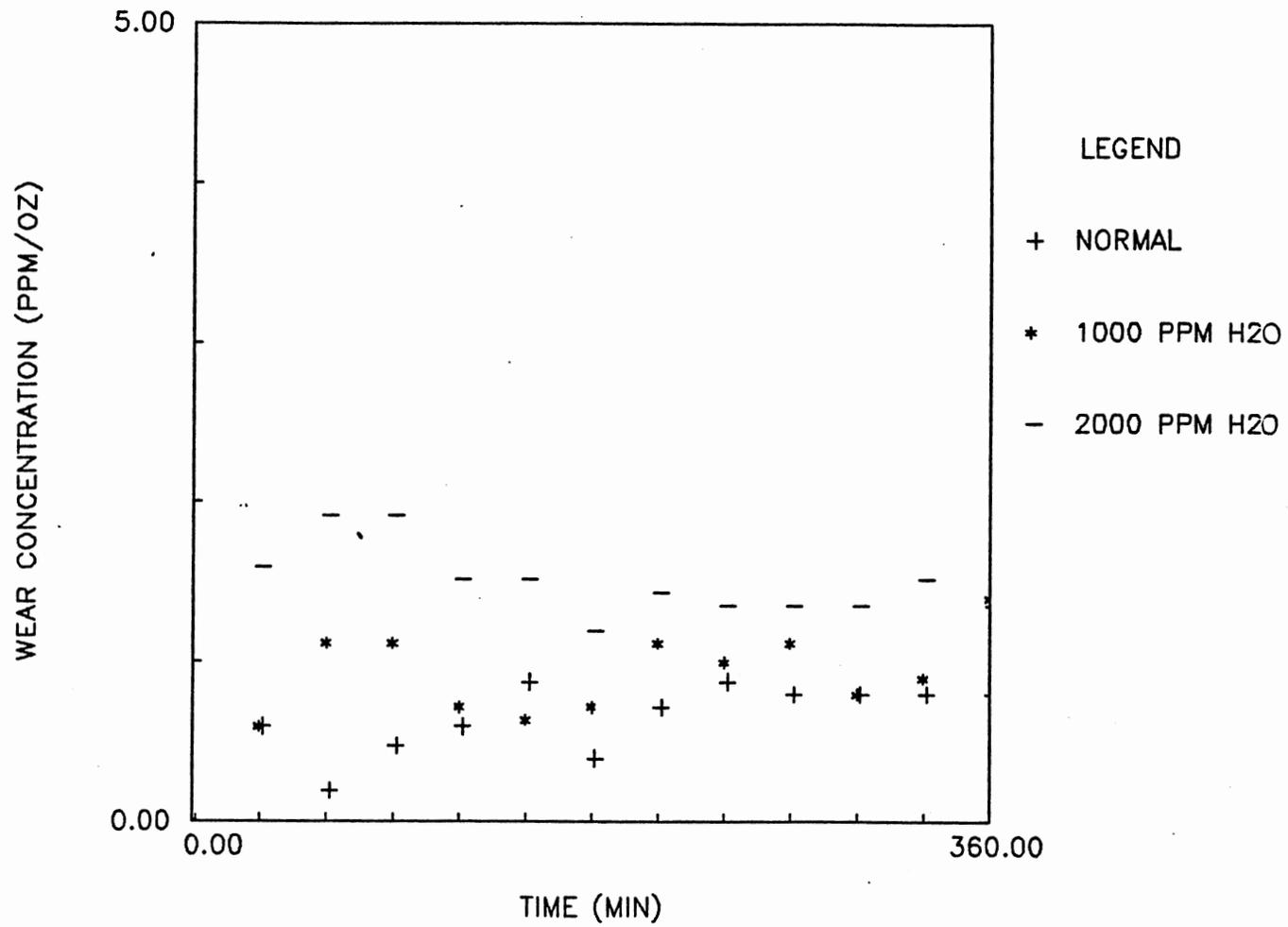
Figure 30. Magnetic wear debris generated under corrosion conditions
