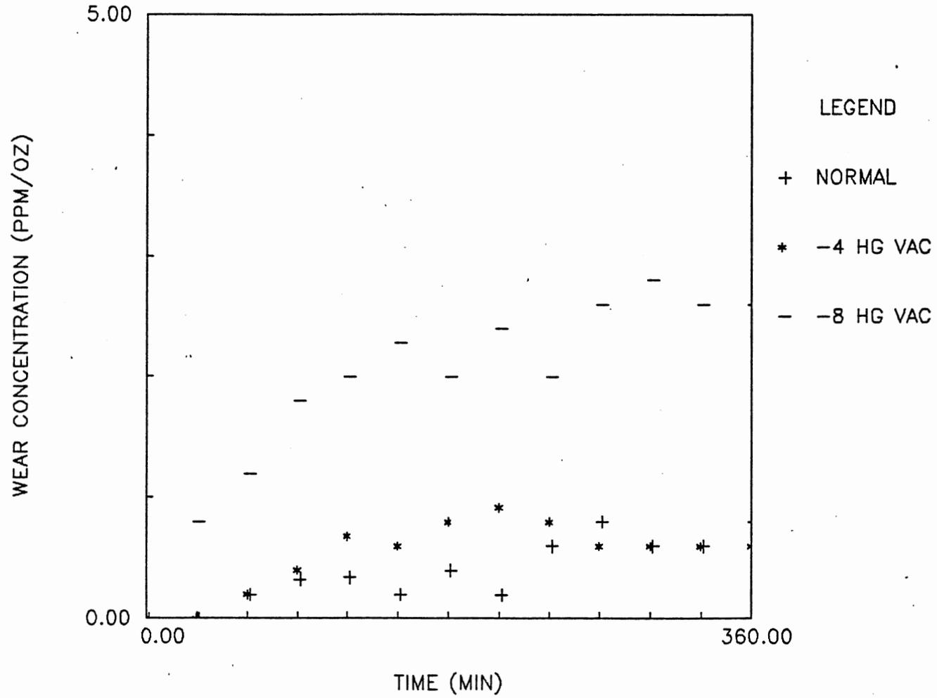
Figure 23. Magnetic wear debris generation under cavitation conditions
