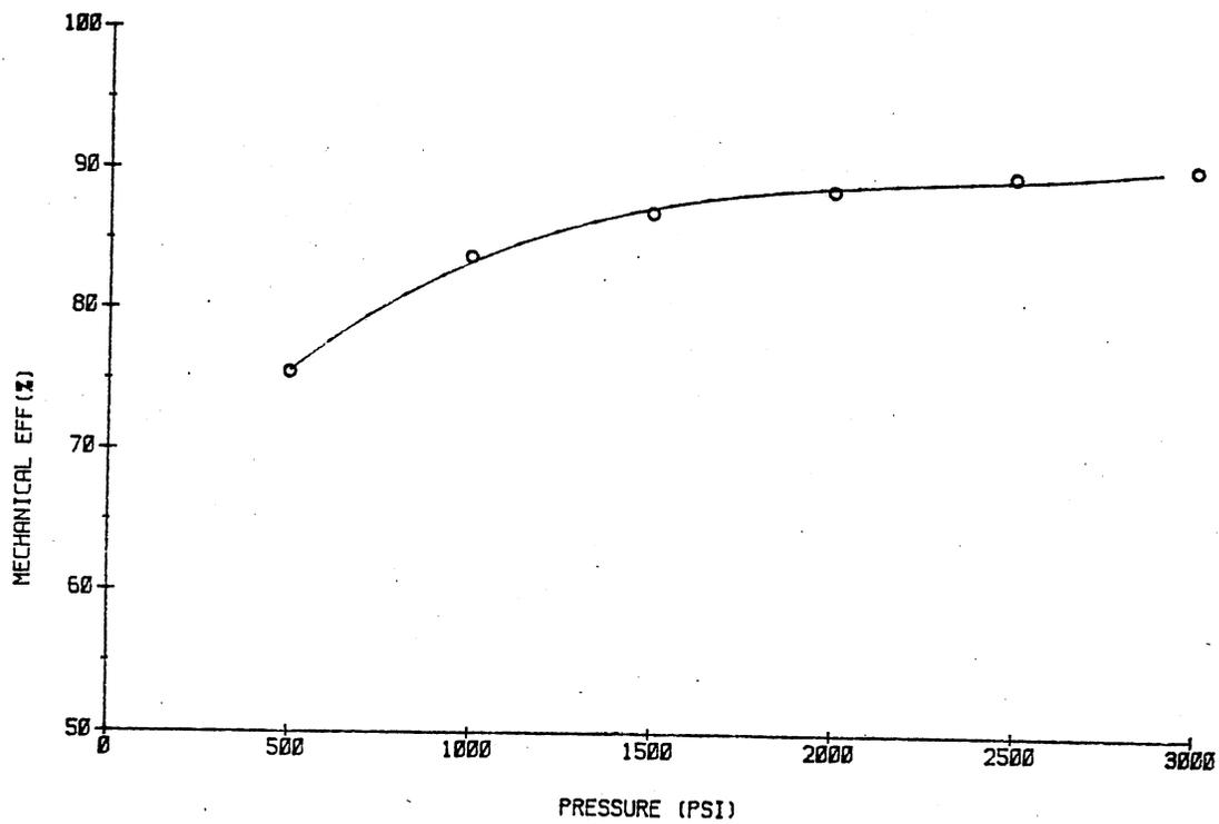
Figure 18. Variation of pump mechanical efficiency as function of system pressure.
