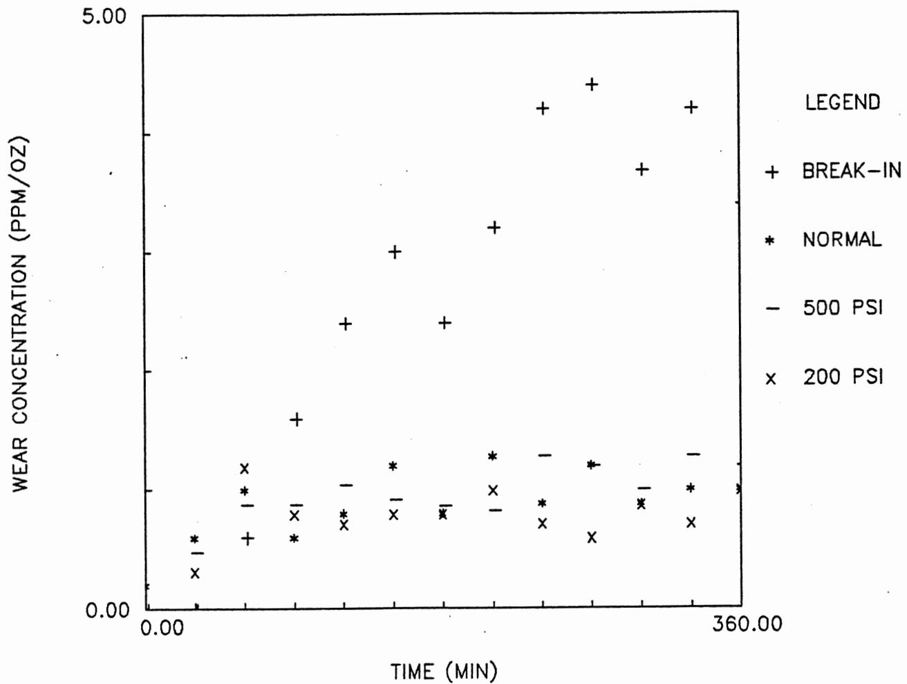
Figure 28. Magnetic wear debris generated under adhesion conditions
