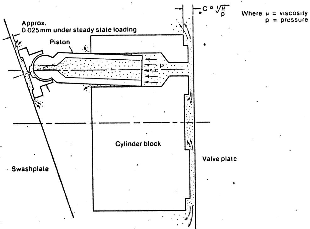
Figure 10. Piston pump clearances
