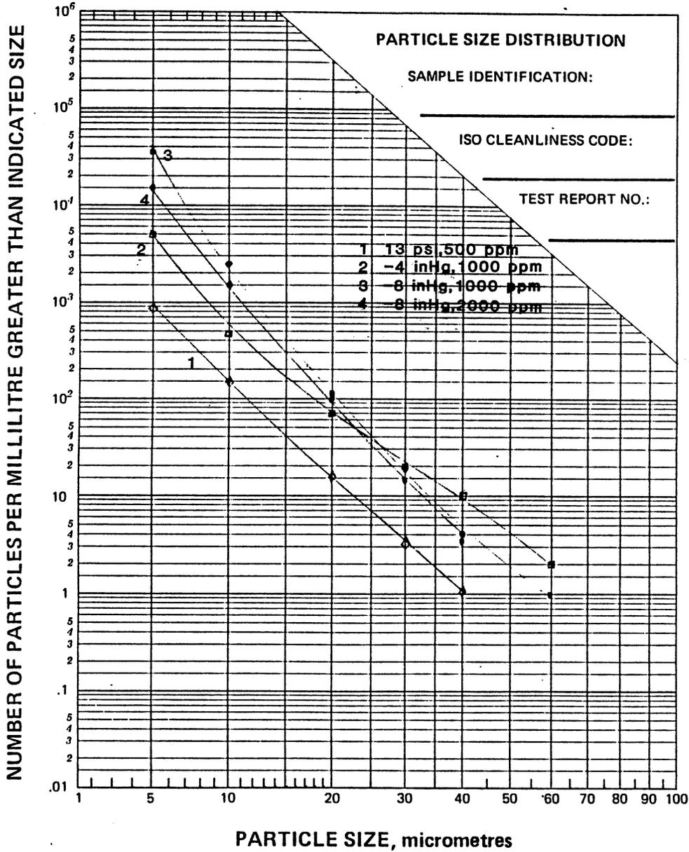
Figure 39. Particle size distribution obtained after six hours of testing. Cavitation-Corrosion wear - Pump 906
