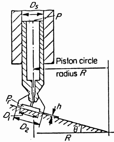
Figure 16. Simplified geometry of slipper path
