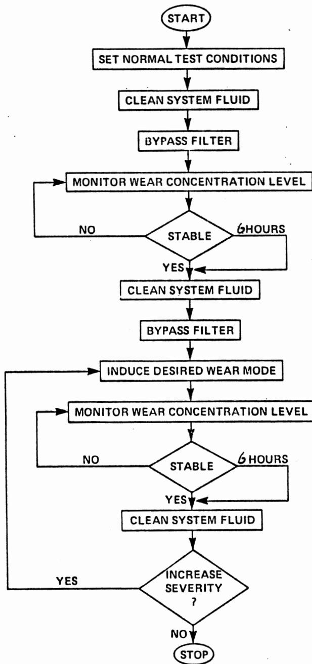
Figure 22. Experimental test procedure
