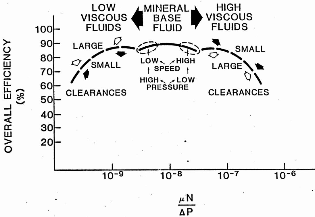
Figure 11. Effects of pump clearances on pump overall efficiency
