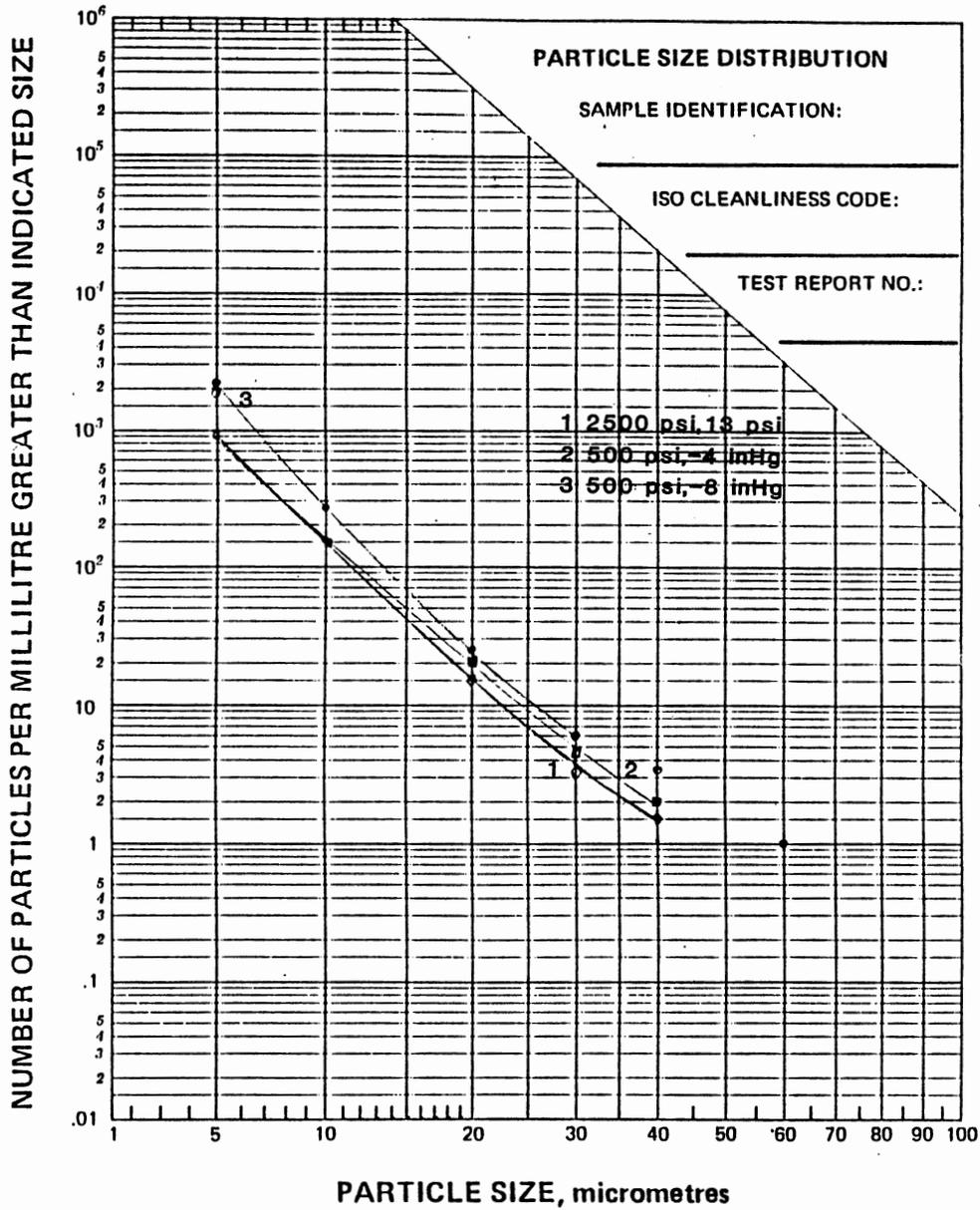
Figure 34. Particle size distribution obtained after six hours of testing. Adhesion-Cavitation wear - Pump 540
