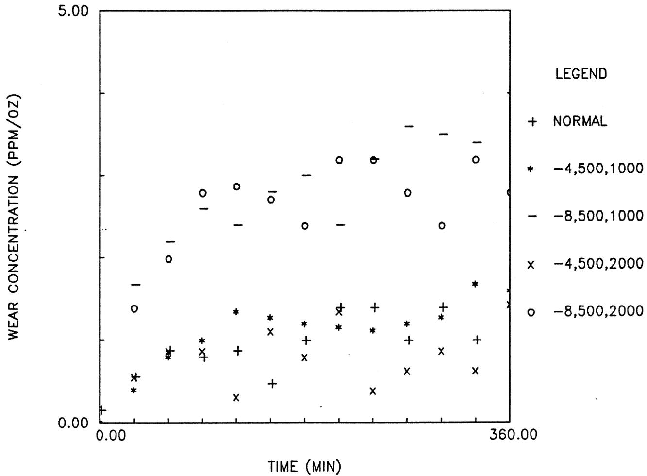
Figure 40. Magnetic wear debris generated under cavitation-corrosion-adhesion conditions
