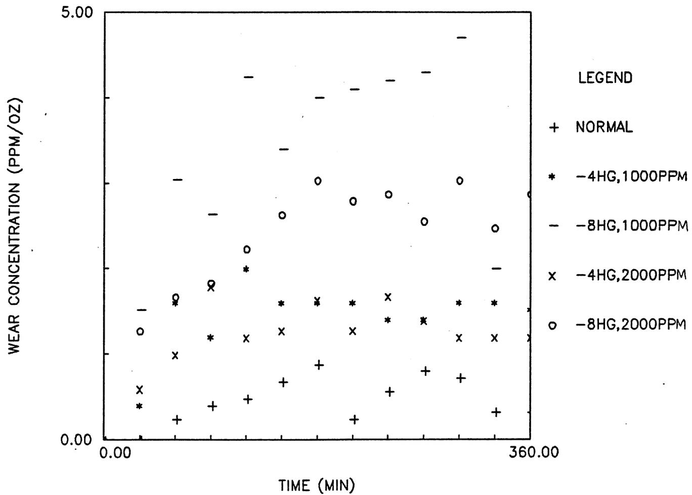
Figure 38. Magnetic wear debris generated under cavitation-corrosion conditions
