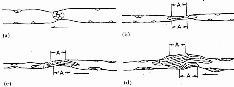
Figure 6. Sasada's model for the press-slide flattening formation of a transfer particle [45]
