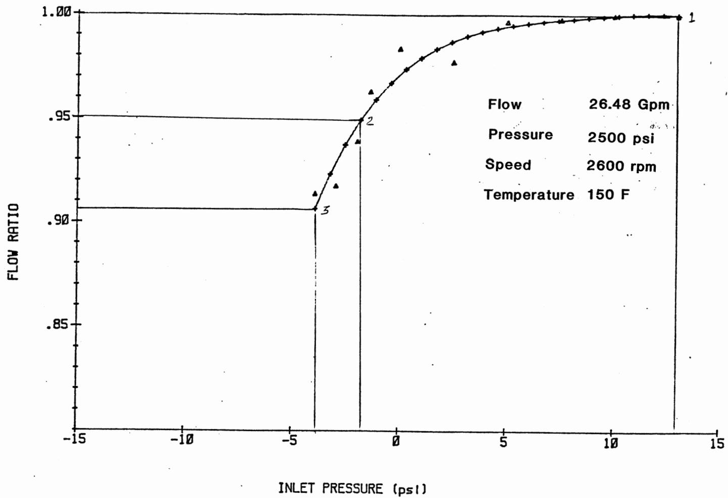
Figure 12. Pump filling characteristic
