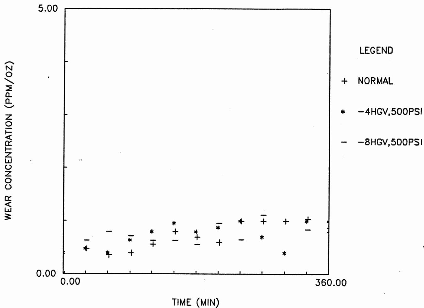
Figure 33. Magnetic wear debris generated under cavitation-adhesion conditions
