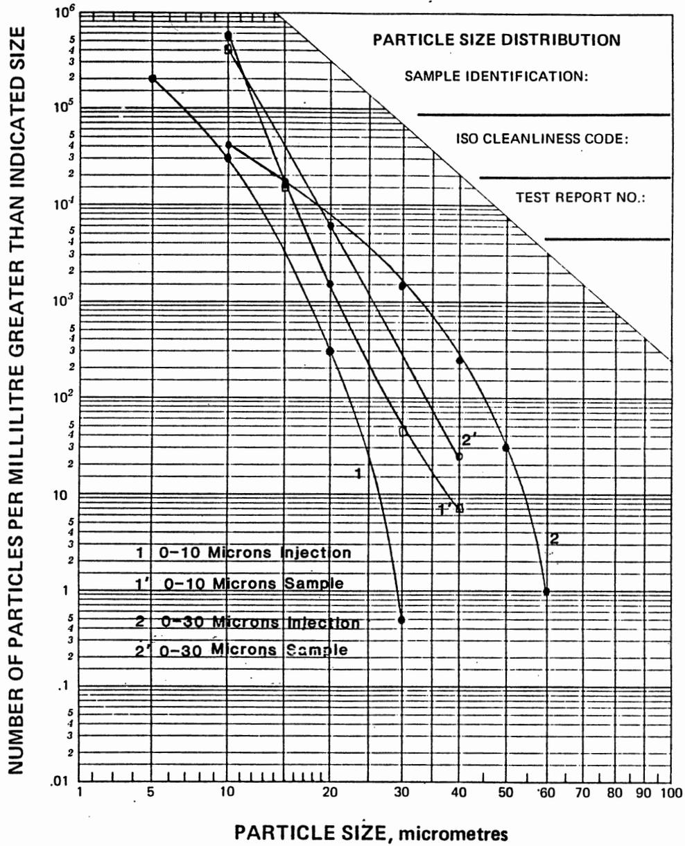
Figure 45. Particle distribution changes after injection in contaminant sensitivity tests.
