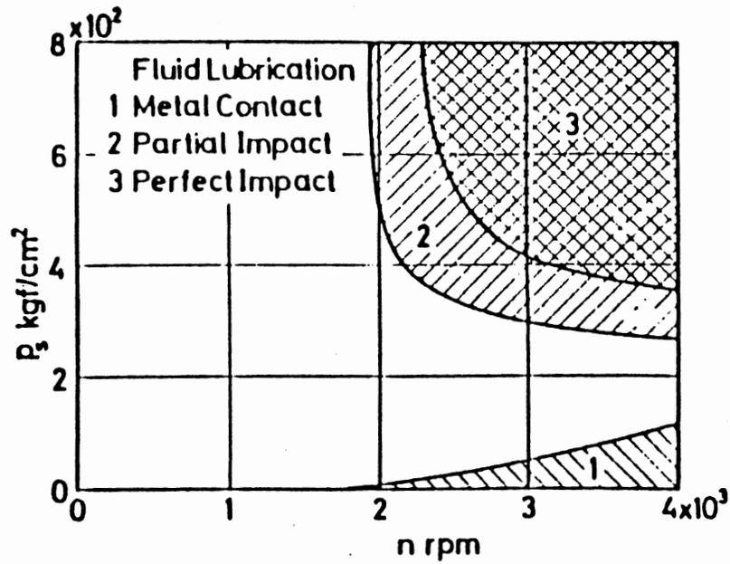
Figure 17. Limit of fluid film lubrication for slipper bearing [59]
