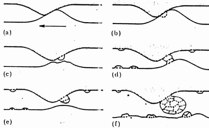
Figure 5. Sasada's model for the formation of a wear particle through a mutual transfer and growth process [44]
