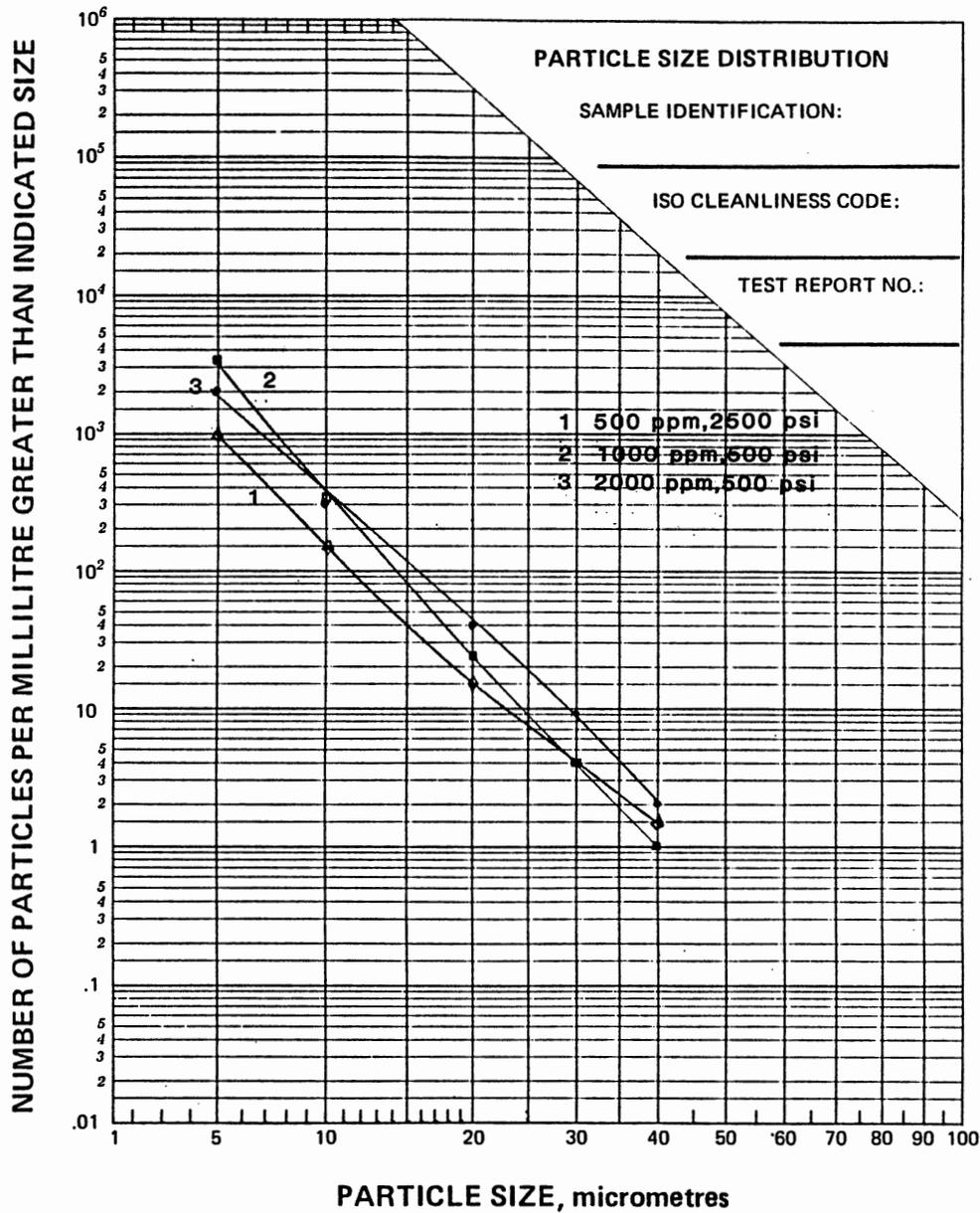
Figure 37. Particle size distribution obtained after six hours of testing. Corrosion-Adhesion wear - Pump 415
