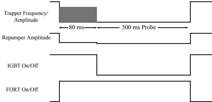
Figure 4.11: Timing diagram for the FORT loading. Gray shading in the trapper timing represents a -15 MHz frequency detuning. After the MOT is loaded for 1.4 s, the MOT trapping laser is detuned by -15 MHz and reduced in power by a factor of 1/3 , at the same time as the repumper laser is reduced in amplitude. At the same time, the FORT laser is turned on. This loading period occurs for 80 ms, then the MOT lasers and IGBT are turned off. The FORT is then probed for 500 ms before the MOT loading cycle begins again.
