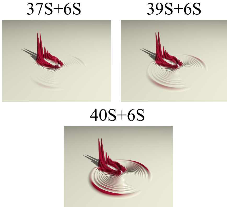
Figure 2.2: Electron probability distributions for the red-detuned vibrational levels of the (37S+6S)^3\Sigma , (39S+6S)^3\Sigma , and (40S+6S)^3\Sigma systems. The ionic core of the Rydberg atom is in the center of the distribution and the ground state atom is at the peak of the portion corresponding to the “trilobite” state. These states have an admixture in the symmetric state, which can be seen in the rings surrounding the ionic core in the probability density.
