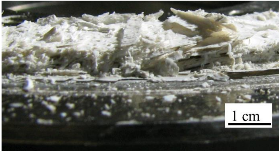
Figure 44. Side view of the dry talc powder sheared at velocity of 0.002 m/s and normal stress of 2.6 MPa for 3.5 m. Note the through-cutting Riedel shears within the talc powders.
