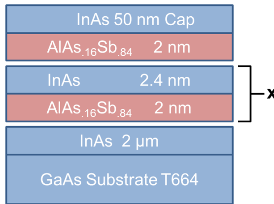
Figure 5.8: A typical InAs SL structure grown to determine the optical properties of the proposed solar cell design. The structures were grown on GaAs(001) 2° off substrates with a 2μm InAs buffer.
