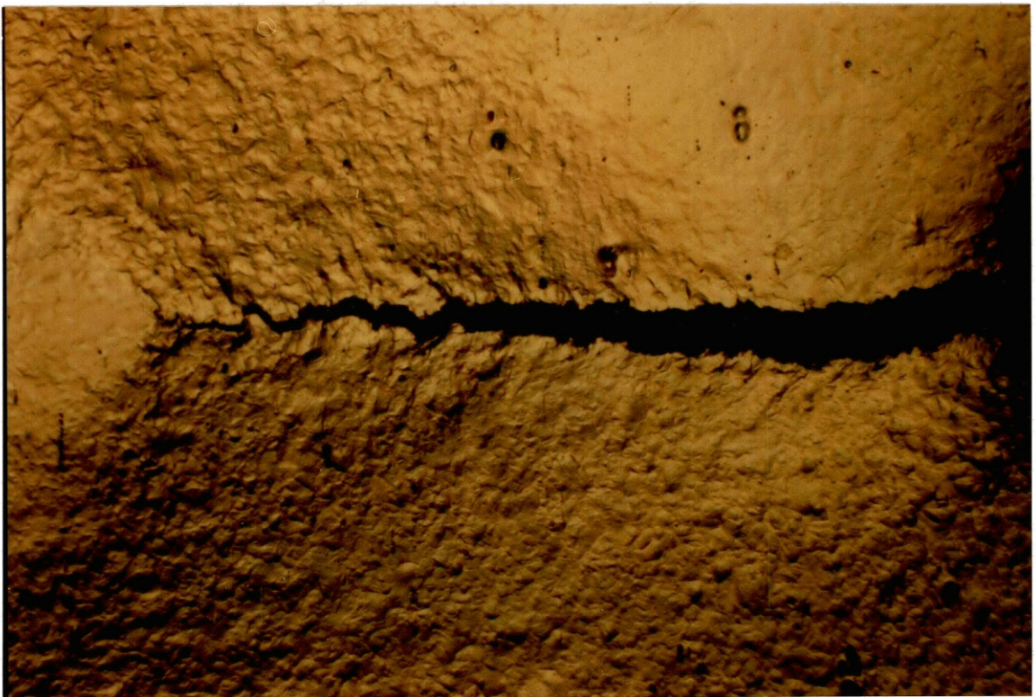
Figure 8. Surface Rumpling Under Axial Fatigue.
