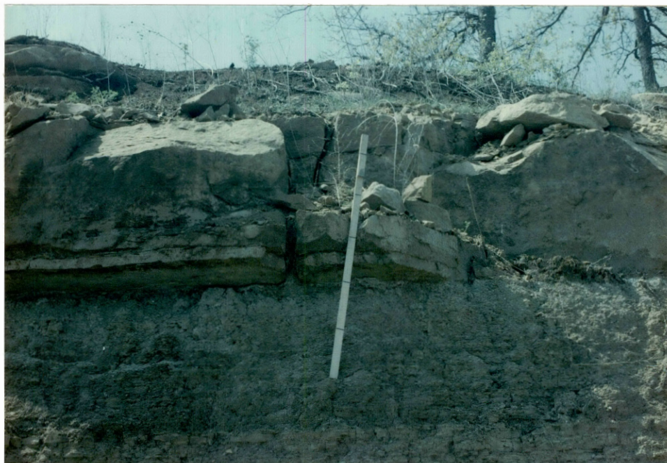
Figure 22: Photograph of a portion of an outcrop in NW/4, Sec. 1, T. 21 N., R. 4 E. showing a jointed sandstone overlying shale. (Jacob staff marked in one foot intervals.)
