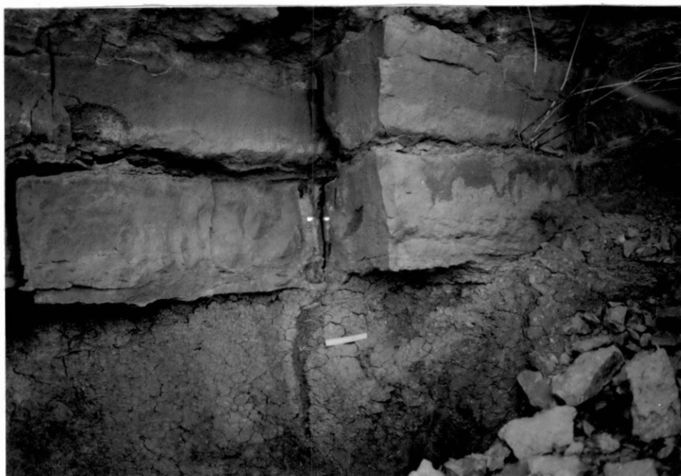
Figure 12: Photograph of a portion of the Oilton outcrop showing the jointed Lecompton Limestone, overlying shale that contains an unrelated set of mineralized joints. (Ruler is 6 inches long.)
