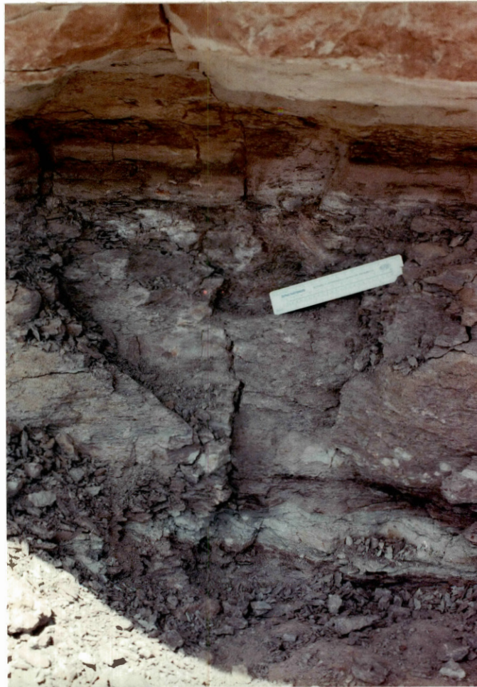
Figure 17: Close-up photograph of rocks shown in Figure 16. Joint passes from sandstone, through shale, into sandstone below. (Ruler is 6 inches long.)
