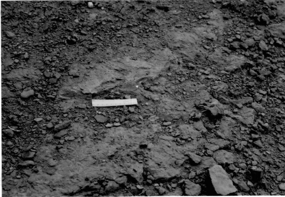
Figure 24: Photograph of the excavated floor of a pit in NW/4, Sec. 1, T. 21 N., R. 4 E. Bleached rock near joints (irregular tan markings) which suggests that joints once have transported fluids. (Ruler is 6 inches long.)
