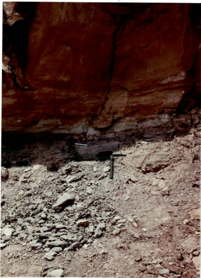
Figure 18: Photograph of a portion of the Ripley outcrop showing a joint that penetrates sandstone and underlying shale. (Camp shovel is approximately 24 inches long.)
