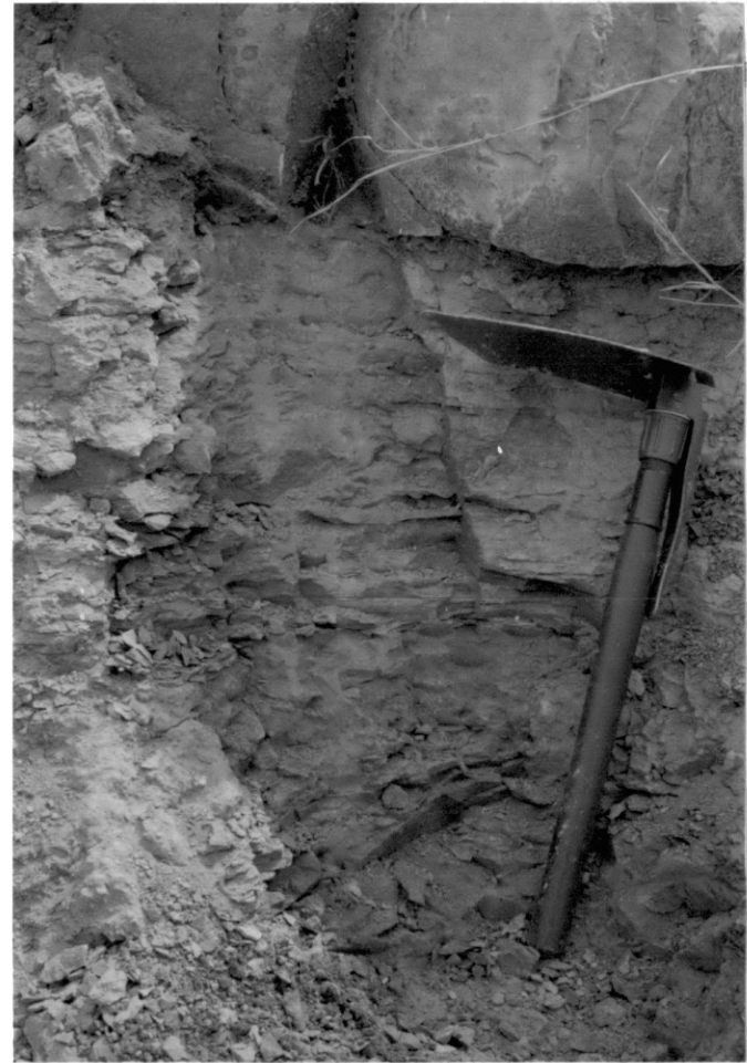
Figure 21: Each photograph shows joints in shale related to joints in overlying competent beds. (Jacob staff showing markings at one-foot intervals for scale in left photograph; camp shovel is approximately 24 inches long in right photograph.)
