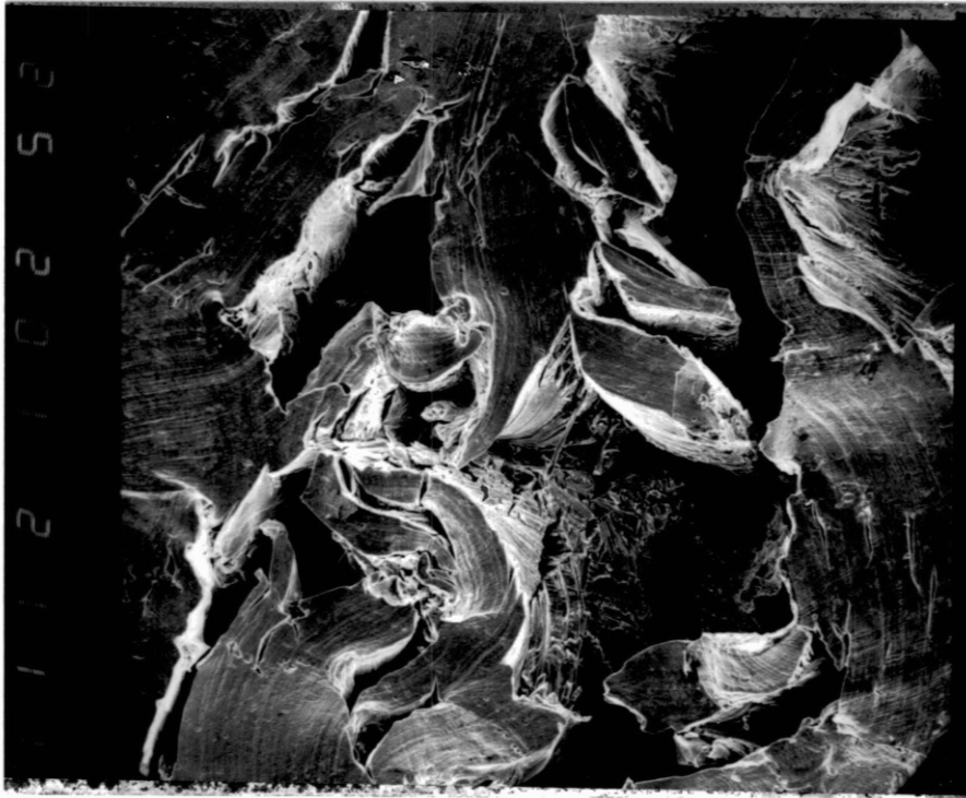
Figure 38. Coarse grain test details of Figure 36, near the fracture. The cracks are gaping under extensive plastic deformation; X 200.
