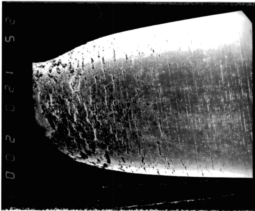
Figure 33. As received Monel 400 specimen, side view of the fracture. Compared to Figure 25, the cracking is less extensive; X 12.
