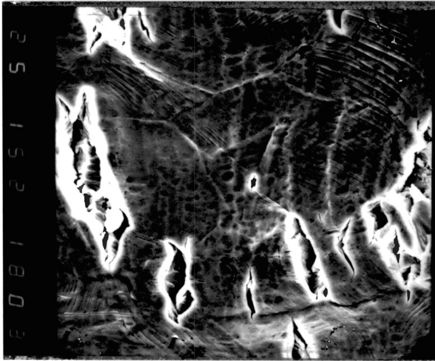
Figure 32. Fast rate test details near the fracture. Smaller cracks, slip bands, and pronounced grain boundaries are revealed; X 1500.
