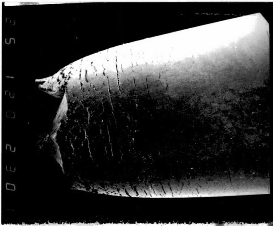
Figure 34. As received Monel K500 specimen, side view of the fracture. The sample is similar to Figure 33 and illustrates less extensive cracking than Figure 25; X 12.
