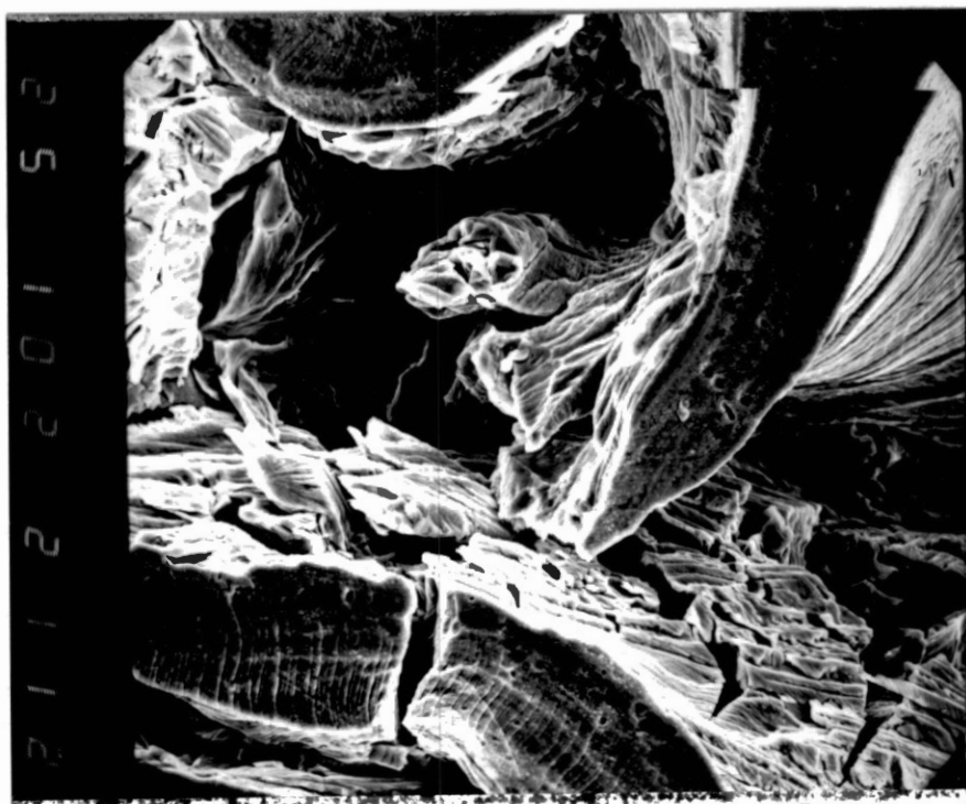
Figure 39. Coarse grain test details of Figure 38. The slip bands, pitting, and diverse nature of TG cracking within gaping cracks are illustrated; X 1000.
