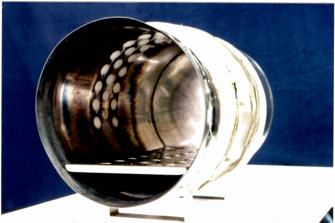
Figure 2: Sterilization Cylinder Used to Aseptically Transfer Supplies Into the Isolator.*
