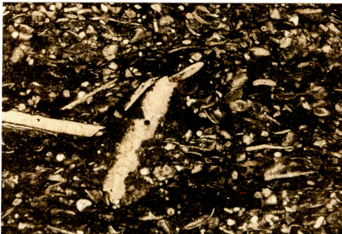
Figure 28. Thin-section photomicrograph showing bedding disturbed by bioturbation, a feature commonly observed throughout Unit 2. From the Kaiser-Francis No. 8-20 Dillard, core depth 5,660 feet. Magnification 40x. Plane-polarized light.
