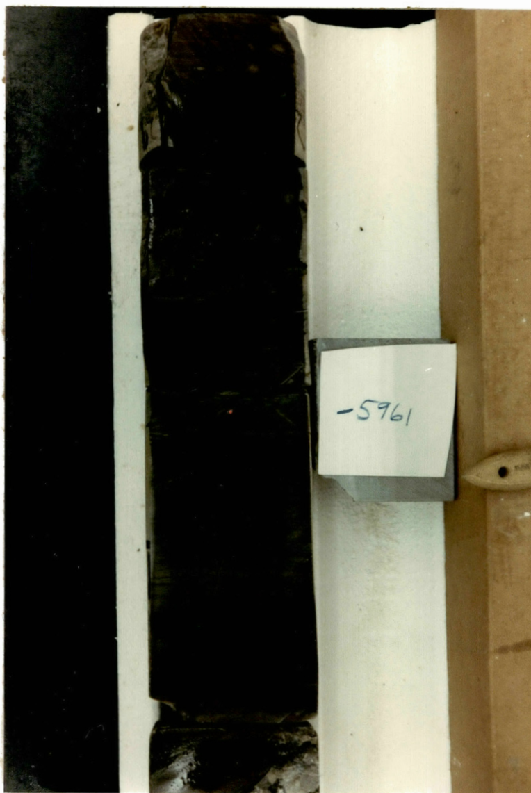
Figure 20. Photograph of Unit 1L. This unit mostly is finely laminated limestone and chert with sparse partings of shale. Light and dark color variation is due to increased amounts of organic matter in the darker horizons. Depth shown is below the surface. Scale of photograph: 1 inch equals approximately 6 inches.
