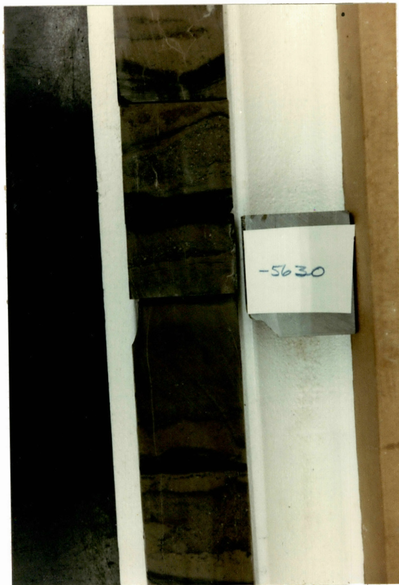
Figure 26. Photograph of a section of Unit 2. This unit is nodular, irregularly bedded limestone. The dark horizontal bands are non-sutured-seam stylolites separating nodules and bedding. Depth shown is below the surface. Scale of photograph: 1 inch equals approximately 6 inches.
