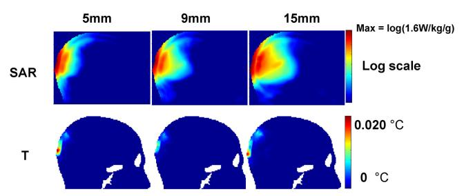
Figure 6. Logarithmic SAR and temperature (T) distributions for the 3 antennas positioned at 0-mm brain depth. doi: 10.1371/journal.pone.0077759.g006
