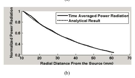
**Figure 3. Electromagnetic power radiation in (a) lossless and (b) lossy media.** (The solid line represents the FDTD calculated data and dotted line represents the analytical data. The power radiation is normalized and is shown as a function of radial distance from the dipole.).
