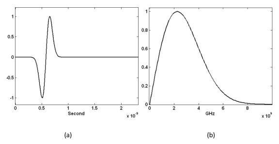
Figure 2. The differentiated Gaussian pulse in (a) time and (b) frequency domains used to power the implanted antenna.
