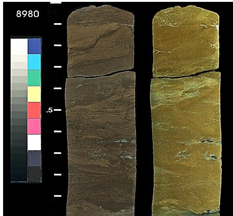
Figure 23: F5 facies from the Mid-Con Energy Operating Hembree 3-17 (Sec. 17 T.6S., R.1W). Deformed laminae in the sandstone are conspicuous. Depth 8980 feet.
