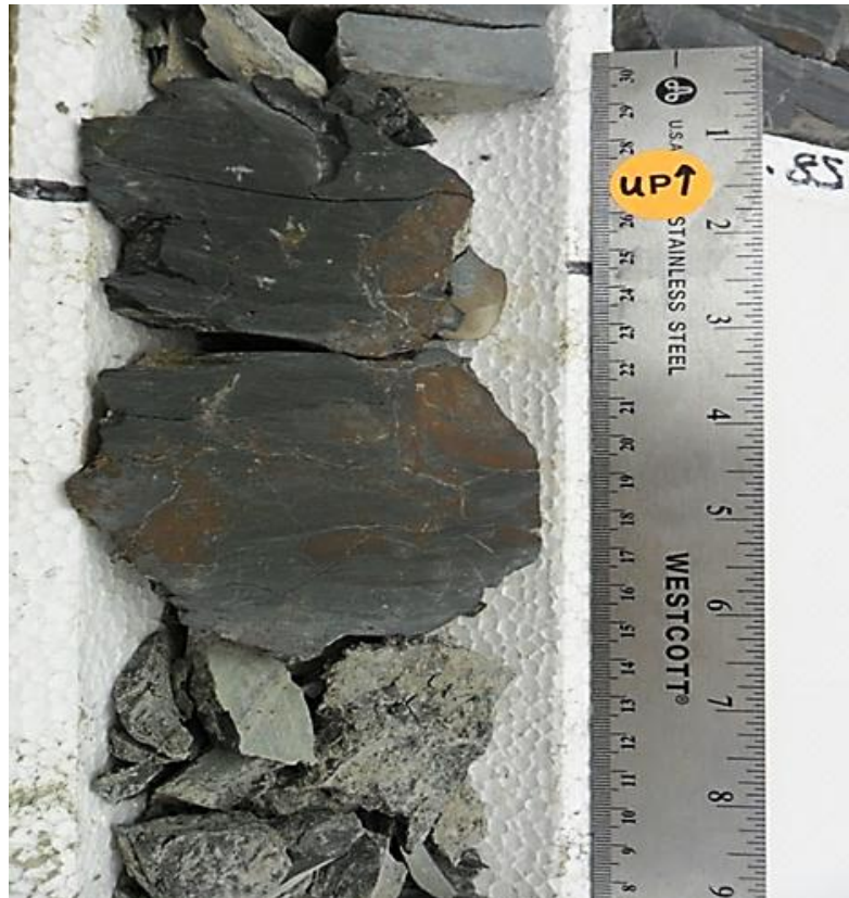
Figure 31: Oxidized zones in the M1 facies from the Mid-Con Energy Operating Hembree 3-17 (Sec. 17 T.6S., R.1W).
