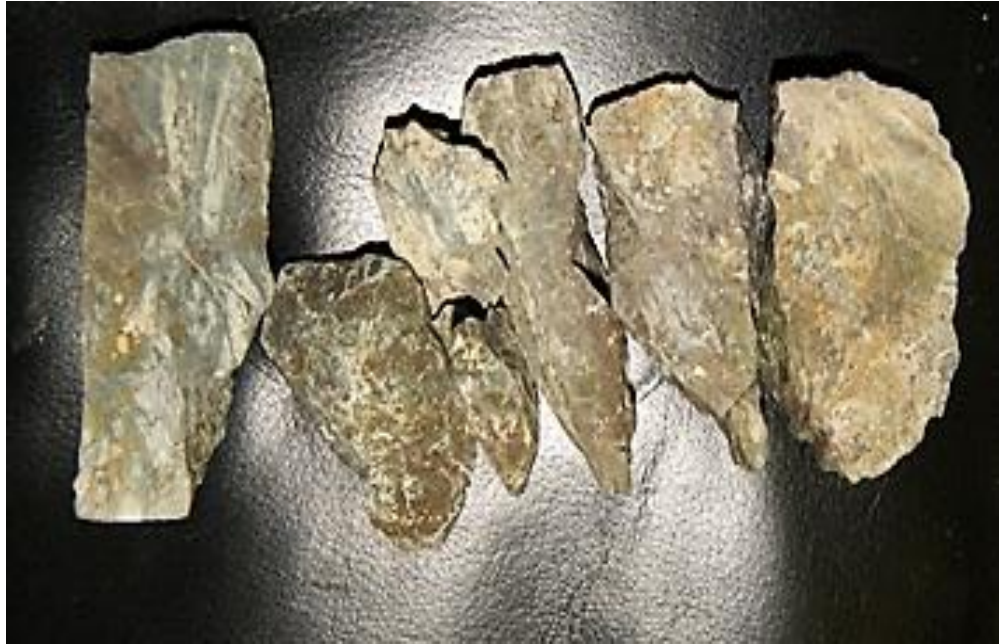
Figure 30: Facies FP from the Santa Fe Minerals, Inc. Gilley 20-2 (Sec. 20 T.6S., R.1W). FP is variegated red-green-grey and has weak structure.
