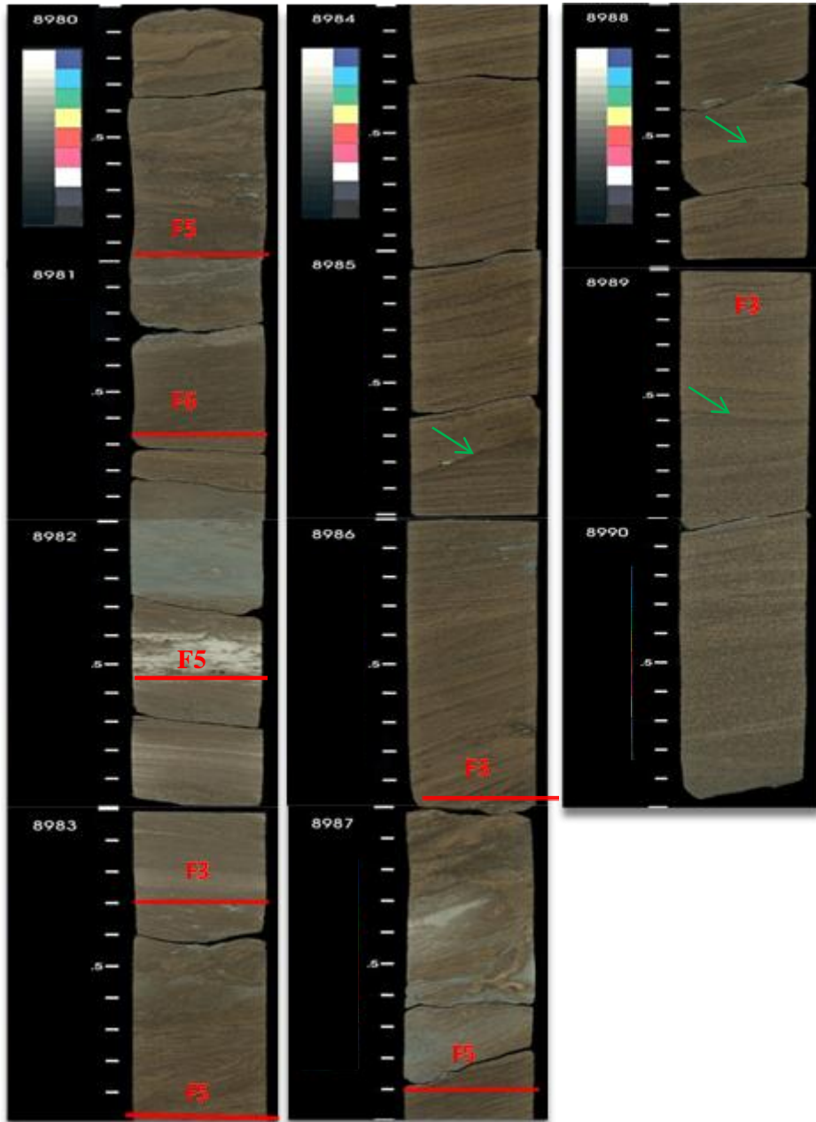
Figure 34: Tussy A sandstone, Mid-Con Operating Hembree 3-17 (Sec. 17 T.6S., R.1W), showing lithofacies, indicated in red. Green arrows point to prominent channel reactivation surfaces. See Table 1 for codes of facies.
