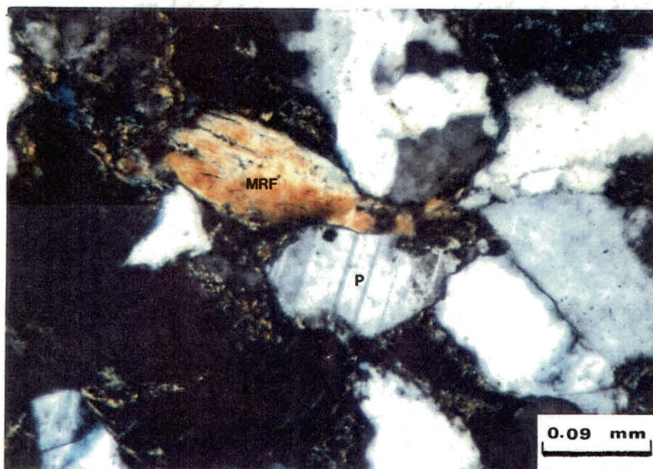
Figure 43. A Microphotograph showing a Plagioclase Grain (P) with the Characteristic Albite Twinning. (MRF): Metamorphic Rock Fragment; Cross-polarized.
