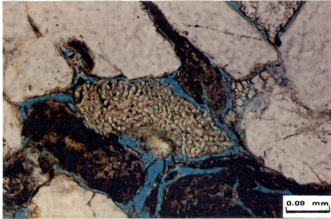
Figure 55. A Microphotograph showing the vermicular nature, the remarkable Coarse Crystal Size and the Worm-like Structure of the Kaolinite Cement (K); Plane Polarized.
