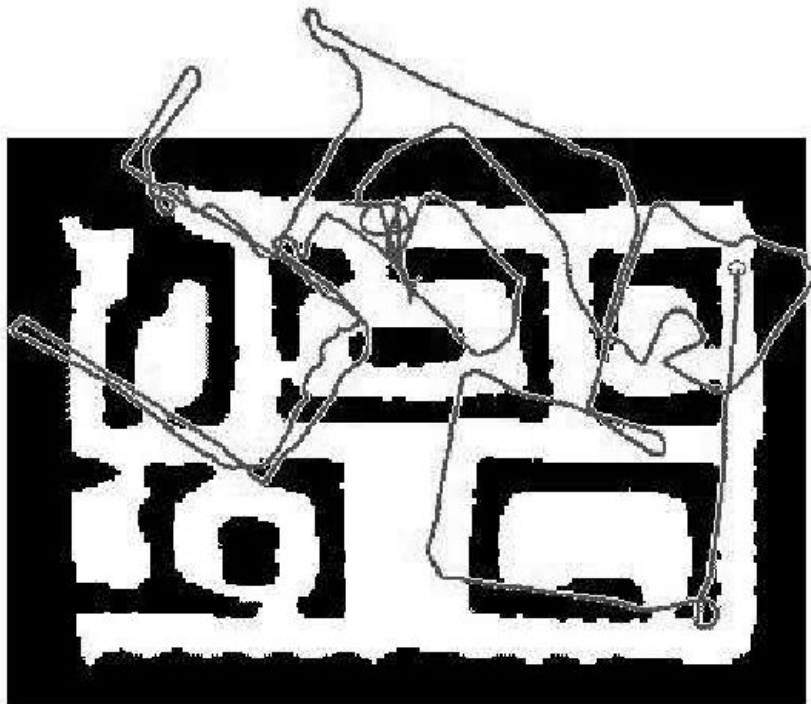
Figure 1.3: A robots path obtained by its odometry, overlaid with the given map. Uncorrected small errors accumulate here. Reproduced from Thrun (2002).
