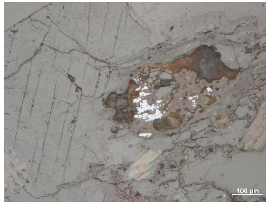
Figure 10: CPL (left) and reflected light (right) photomicrographs of reddened Dalradian schist in Scotland. The hematite is seen altering pre-existing grains, likely biotite.
