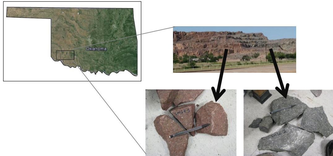
Figure 2: Long Mountain Granite quarry, located in the Wichita Mountains of southwest Oklahoma. The inset picture shows the red granite at the surface (left) and the green granite (right) exposed by quarrying operations.
