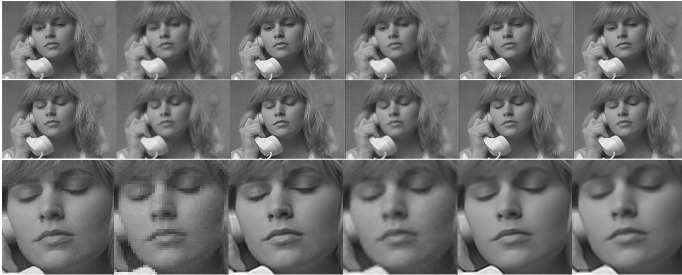
Figure 2.9: Video super resolution for Suzie sequence: (frame 28 and 18 with the resolution ratio 3, PSNR in brackets). From Left column to Right column: Ground truth; LR frame; GNL-Means [2] [PSNR: 29.87 - 29.86]; Lanczos interpolation [3] [PSNR: 29.41 - 29.27]; SCoBeP-NLM [PSNR: 30.95 - 30.75]; SCoBeP-SR [PSNR: 30.55 - 30.71].
