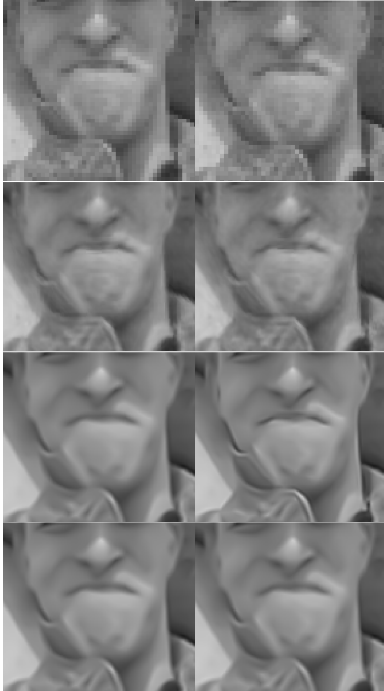
Figure 2.13: Video super resolution for Foreman sequence with noise: I added synthetic additive white Gaussian noise (AWGN) to the input LR sequence, with the noise level \sigma_n = 1.20 (left) and \sigma_n = 2.00 (right). From top to bottom column: Noisy LR; 3-D ISKR [4]; SCoBeP-NLM; SCoBeP-SR.
