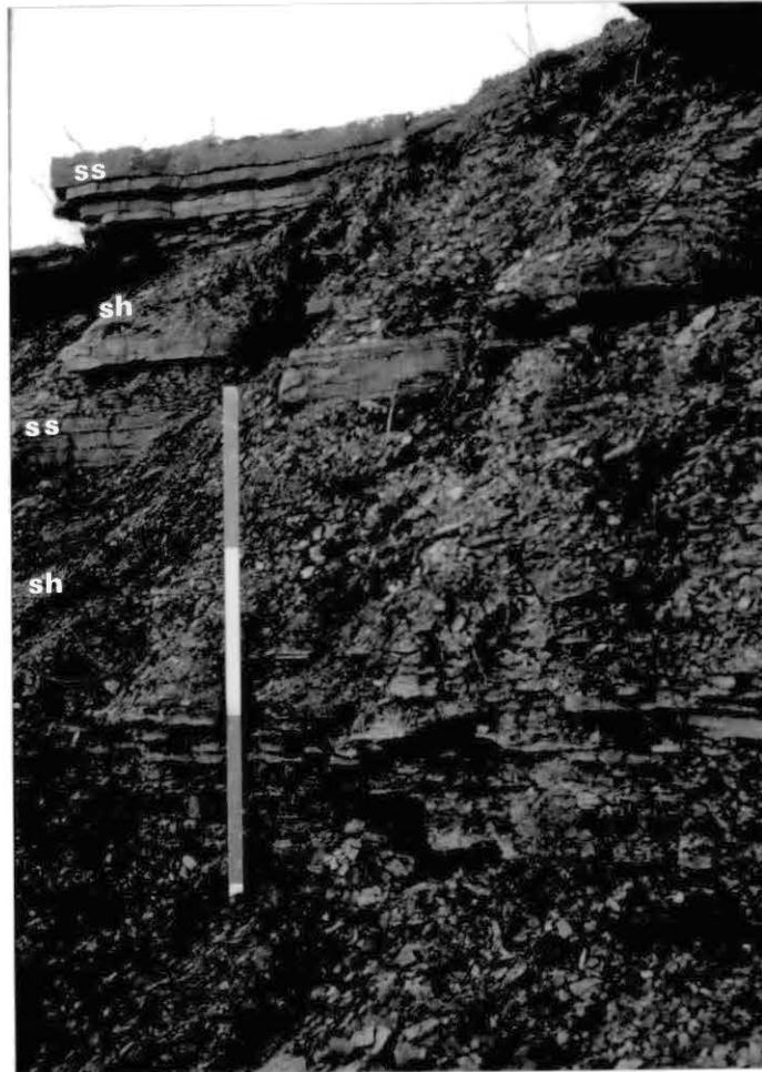
Figure 7. Outcrop of Nellie Bly Shale with Thin Interbedded Sandstones - West 1/4 Corner, Sec. 28, T. 24 N., R. 13 E. (Jacob Staff 1.5 m).
