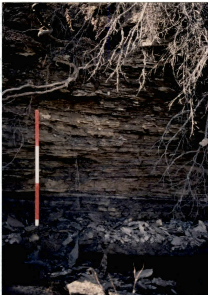
Figure 12. Alternating dark gray-to-black shales and thin-bedded sandstones - NE 1/4, Sec. 33, T. 21 N., R. 11 E. (Jacob Staff 1.5 m).
