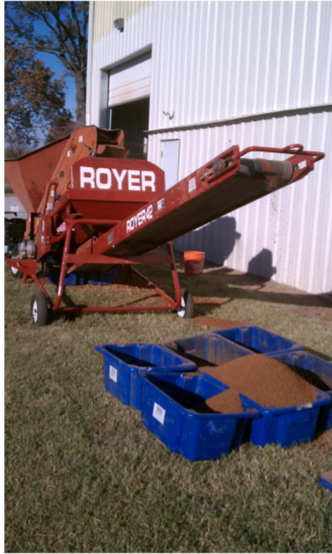
Figure 4.6. Soil processing for reduced-scale embankment tests using a crusher-sifter machine
