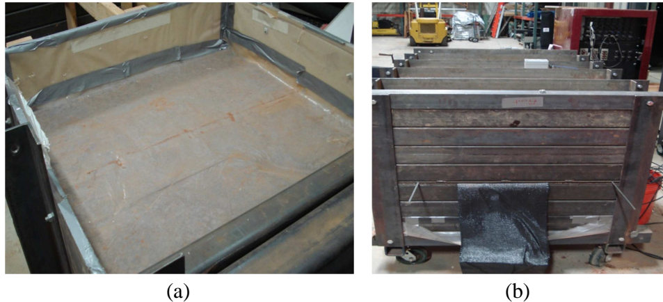
Figure 3.9. (a) Sealed compacted soil at the end of large-scale pullout box setup, (b) Geotextile specimen at the mid-height of the pullout box
