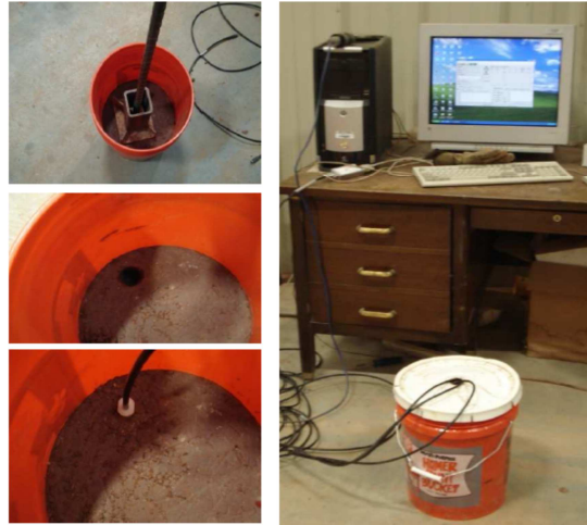
Figure 6.1. Fredlund sensors placed in a calibration bucket to measure matric suction of the Chickasha soil
