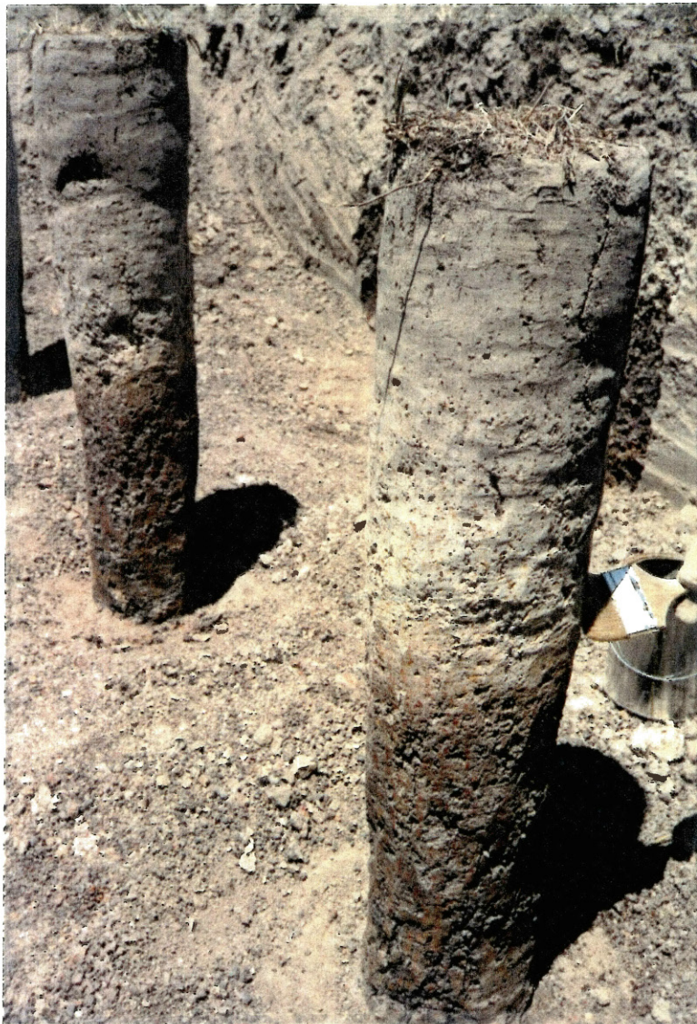
Fig. 7. Stigler soil as a free standing column.
