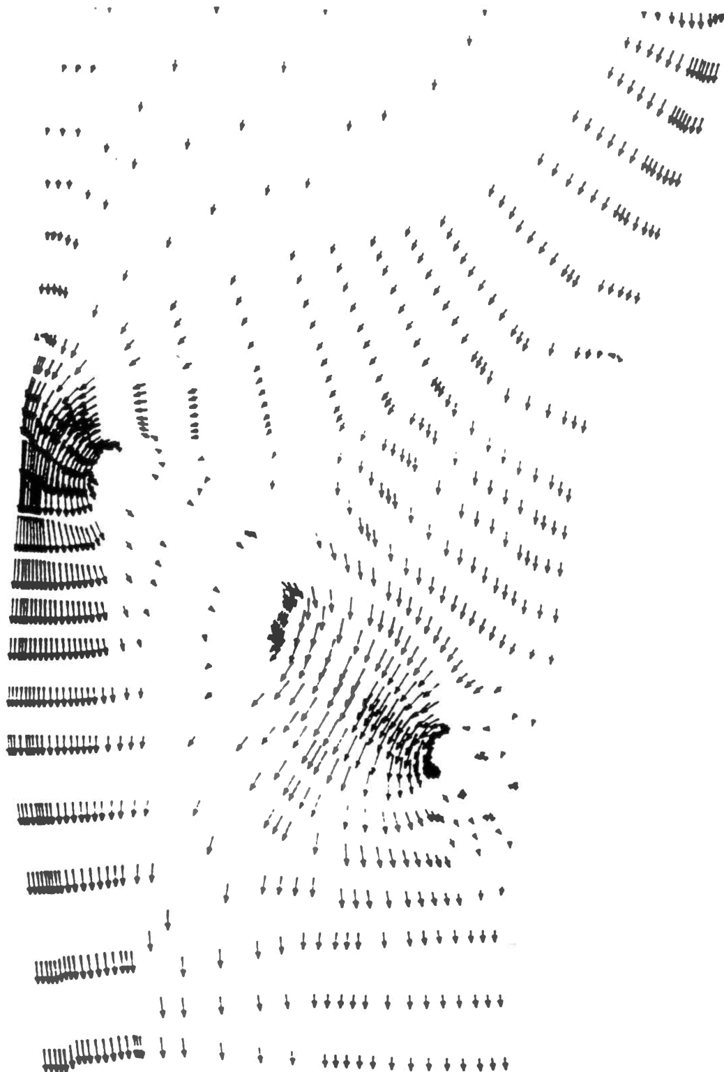
Figure 13. Velocity Vectors for Q_{1,mn} . Scale 1"=35.0 fps
